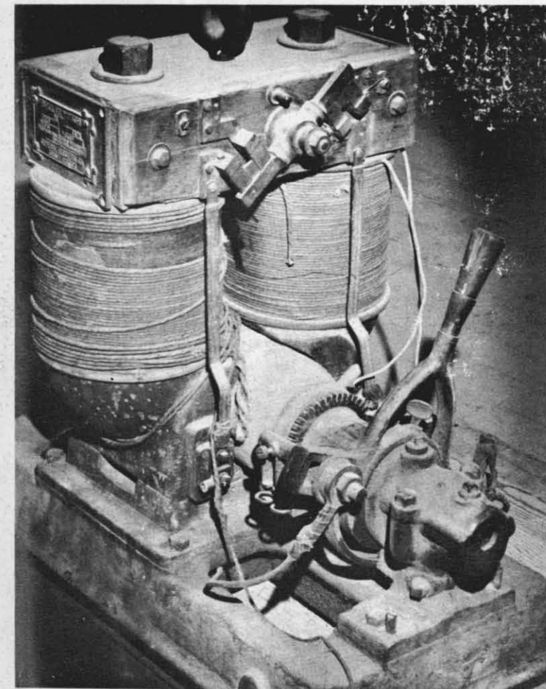
LITTLE WORKHORSE OF STANDARD MILL —This is one of the first electric motors to operate by long distance power in the industrial world. It received its "juice" from the Green Creek hydroelectric plant 13 miles from Bodie, and ran the gold ore stamping system in the Standard Mill. A plate on the side of the motor reads: Bipolar Motor—NO. 1092-3 KW—500 Volts -- Patented Dec. 23, 1879 -- General Electric Co., Edison System. Engineers were convinced that the transmission lines must be straight since the current might jump off on a curve.
