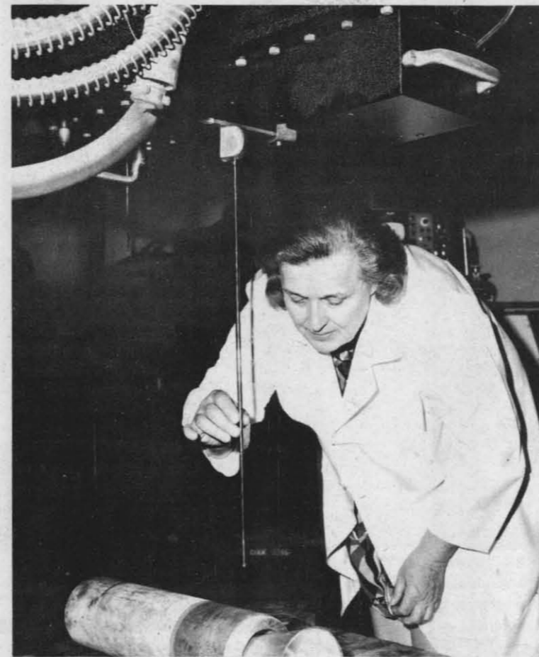
ANN NORWOOD, of the non-destructive testing laboratory, uses a 250,000 volt X-ray to examine a piece of hardware to determine its porosity or cracking of a weld.
