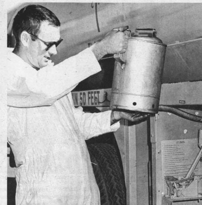
MAC McCarty services a pump engine on a refueler. Maintenance and service is performed on all equipment on the Center with a Navy number by the Transportation Division.
