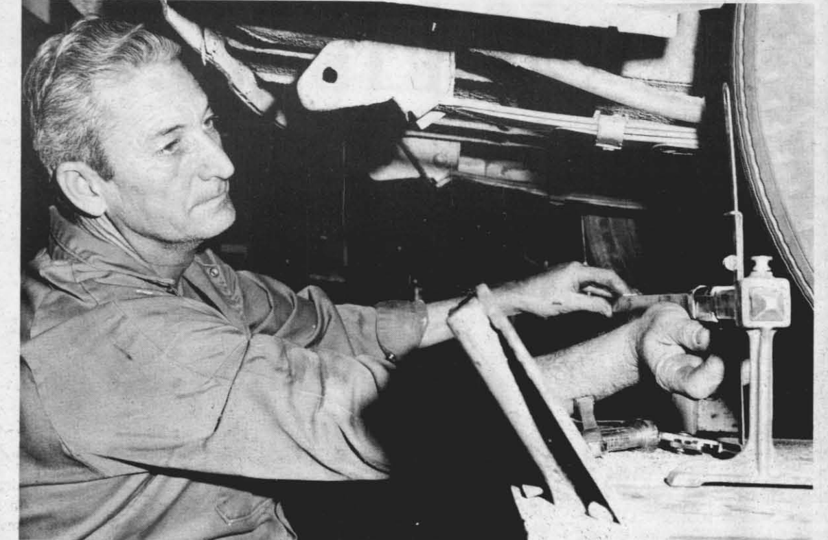
JESSE LEWIS aligns the front end of a half-ton pickup in the automotive shop. Lewis, who performs all types of maintenance, is known in the shop as a radiator specialist.
