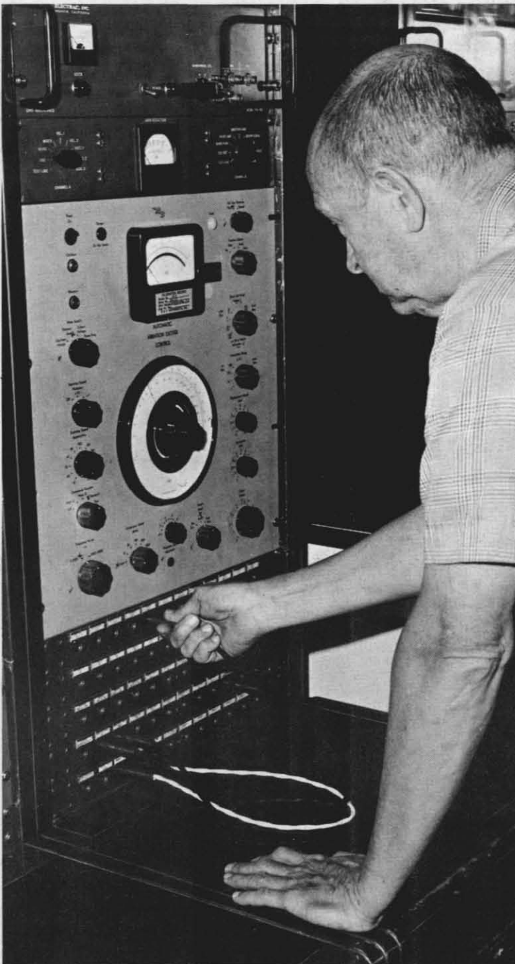
MITCH THORNGATE programs electrodynamic vibration system for random wave evaluation of missile guidance section. The dynamic environments (vibration, shock, and acoustics) are the most difficult of all environments to simulate in the laboratory. Thorngate will use more than 50 instruments to synthesize and control the required random vibration inputs. Code 55171 performs experimental and developmental dynamics tests on items ranging from a miniature transistor to a full scale missile.
