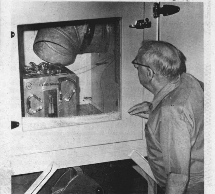
HAROLD MUNN examines Condor pressure sensors which are undergoing a combined vibration-temperature test. The sensors are being vibrated with an electrodynamic exciter capable of producing vibratory forces of 15,000 pounds. Similar tests can be performed with five other Code 55171 vibration systems.
