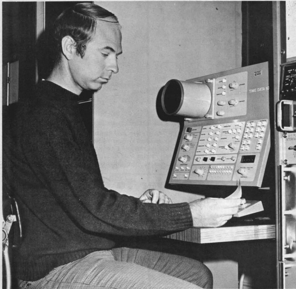
RON BACKMAN programs digital analyzer for spectral evaluation of acoustic data acquired during recent Shrike flight test. The Time Data Analyzer performs real time and delayed time analyses of both analog and digital information acquired during evaluations.
