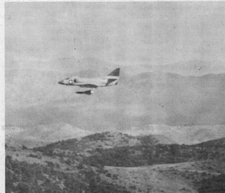
WALLEYE FIRING - AOD received complete responsibility for the development of the Walleye weapon in 1963. The weapon, a television-guided system designed to home on visually acquired targets, was released to the fleet in 1967. The system was a direct result of feasibility studies that were begun by AOD in 1959.
