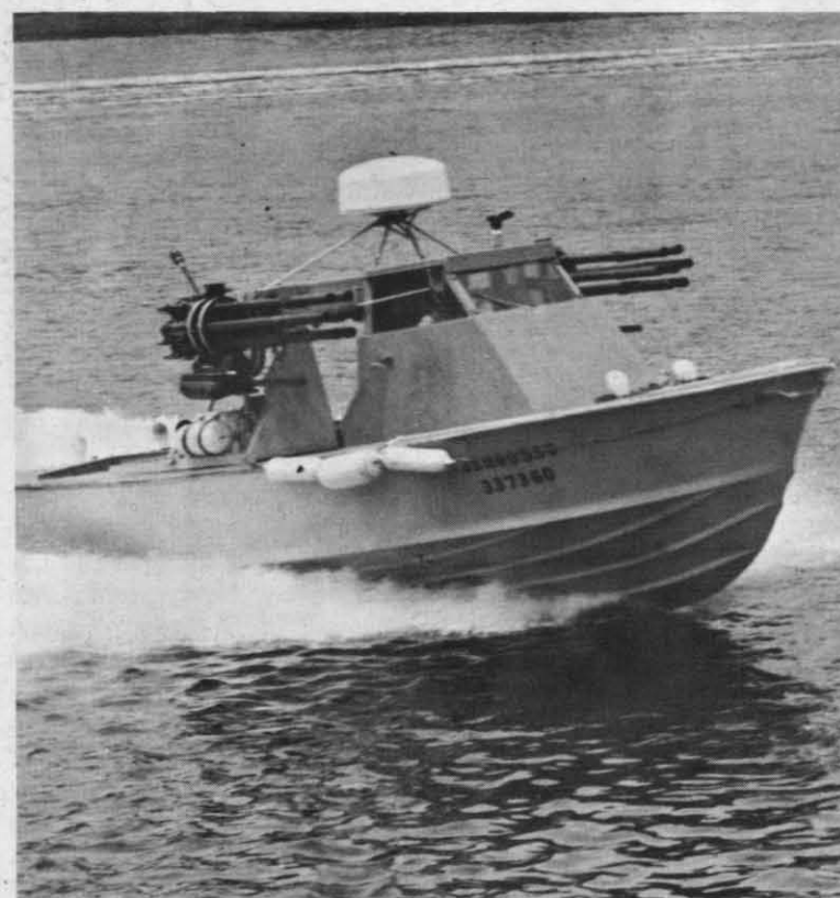
SWAB - The Shallow Water Attack Boat (SWAB) was developed by the department in 1964. An experimental device, the craft is designed to be deployed in areas requiring coastal interdiction.
