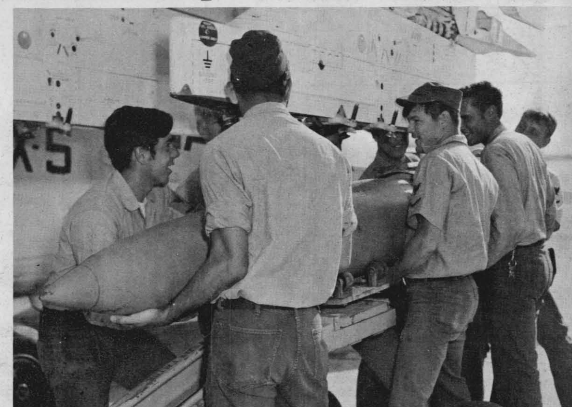
AN ORDNANCE CREW loads a 750-lb. bomb aboard an A-7 for a live ordnance test. Approximately 85 per cent of all VX-5 flights carry either live or dummy ordnance for used on the test ranges. The A7E allows a pilot to strike in any weather.
