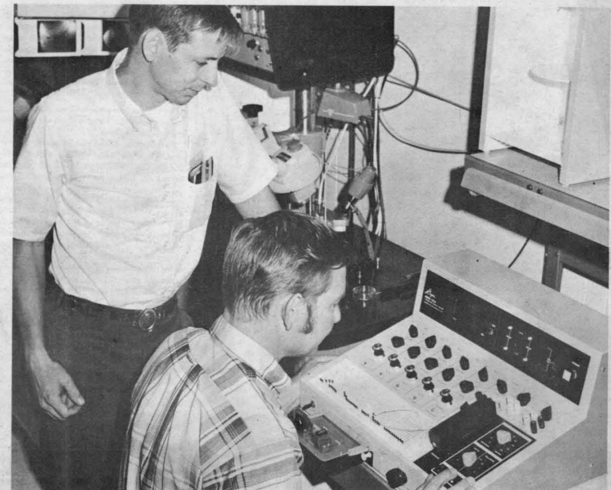
MICROELECTRONICS EFFORT—One of the occupants of the new Solid State Devices Facility will be the Microelectronics Branch of the Engineering Department. Above, Richard Tolkmitt, Microelectronic Technician, operates an integrated circuit tester in the group's present spaces as Branch Head Henry Blazek looks on. The tester is one of several test and analytical instruments for electrical parameter evaluation that will be put to use in the new laboratory. —Photo by PH2 D. E. Hart
