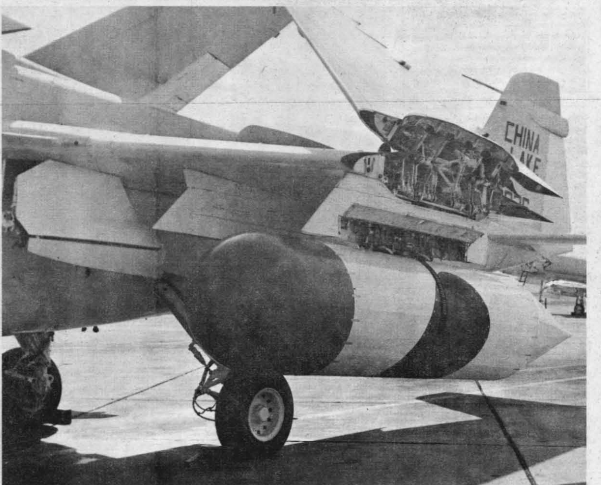
NEW RADIOMETER — A high-resolution, wide-angle microwave mapping radiometer, operating at Ka-band, has been developed by the Center's Corona Annex. The solid-state miniaturized system is used for terrain-mapping. (See page 3 for more details.)
