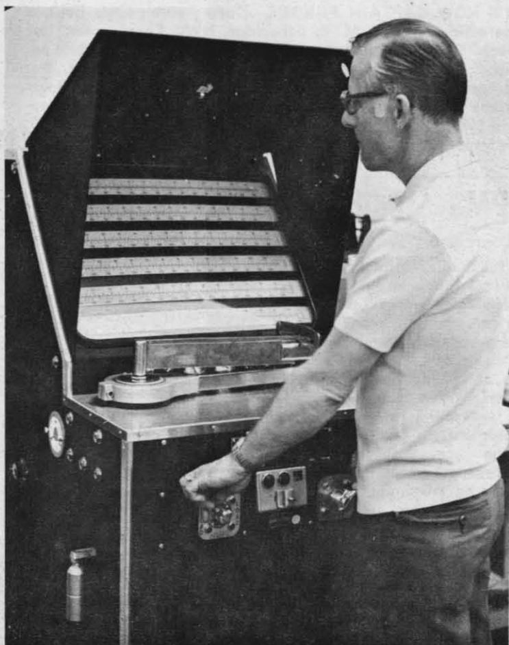
HOWARD GRANT calibrates a torque-wrench with a torque tester which measures from 0 to 1980-inch pounds.
