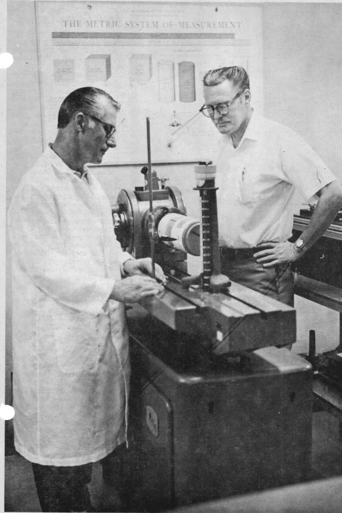
STAN BJORK calibrates gage blocks with a Micro AC machine, which measures lengths within 1 millionth of an inch. Bill Kummings, Head of the Quality Assurance Branch, Engineering Department, watches the operation.
