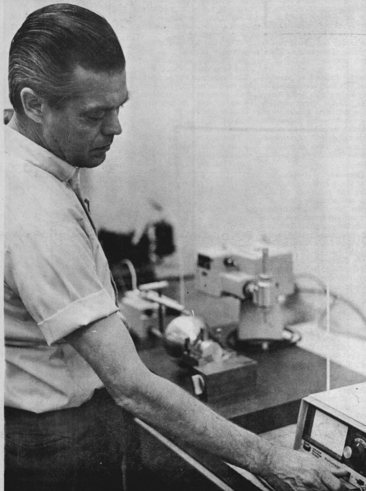
TOP LEFT—Bobby Kochman operates a Lead Tester, which is used for testing thread gages in the realm of 100 millionths inches tolerance.
