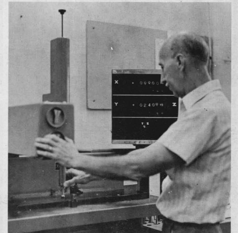
ENOCH NICHOLSON measures a hole pattern on a metal part by using a Cordax 3-dimensional measuring machine. The machine has an accuracy of .0002 inches tolerance.
