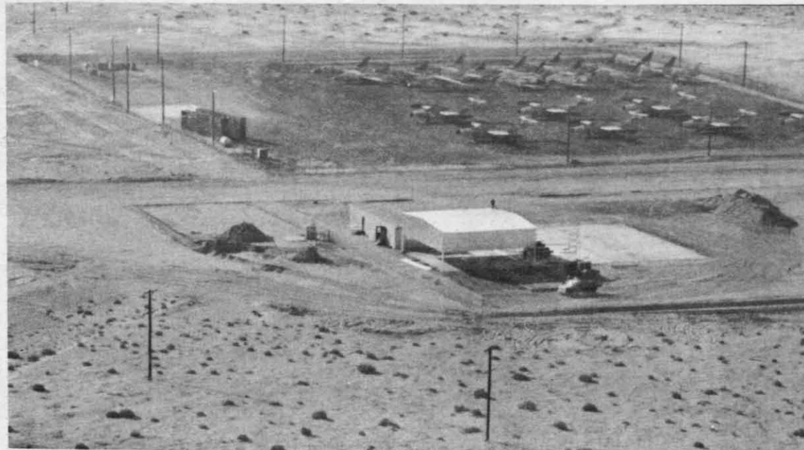
AIRCRAFT SURVIVABILITY COMPLEX —Pictured in foreground is the compound which includes the instrumentation building and pre-test checkout pad for full-scale aircraft and their instruments, target systems, and engines. In the background are F-89, F-86, and A-4 test aircraft which represent the type aircraft that will be used to gather data for the program. The six-acre area provides parking for 35 aircraft and storage for portions of airframes, structural parts, components & bulk spares.
