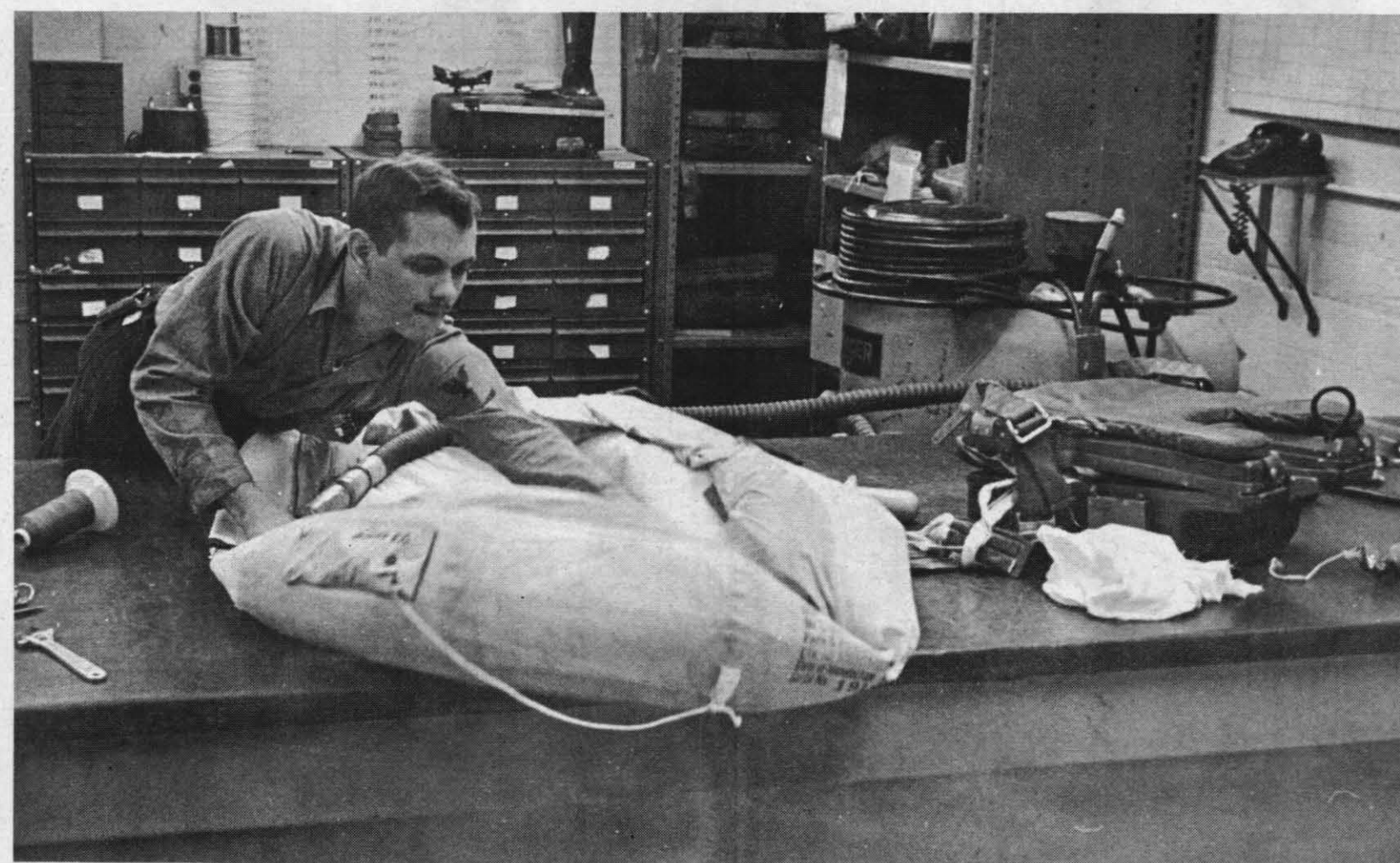
ABOVE—PR3 Ronald Buchanan, of the Raft Shop, a part of the AMD Aviators Equipment Division, deflates a LR-1 Life Raft prior to checking it by inflating it to 2 psi for a 48-hour period. The Raft goes into the container on the right. After being packed, the chute is a part of the ejection seat and is ejected with the pilot in case of an emergency. BELOW—PR1 Fred Mackal (foreground) and PR3 Tom Parrish drop a chute from the drying tower in preparation for repacking. The men in this shop are responsible for the repack and modification of all types of parachutes and life rafts used in both reciprocating and jet aircraft. PR1 John Malan is the Shop Petty Officer.
