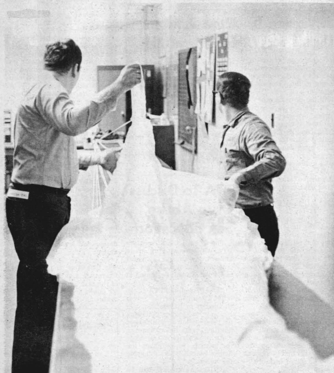
ABOVE—PR3 Ronald Buchanan installs a life raft after having run a 48-hr. check on it by inflating it to 2 psi for the time period. The chute, which is ejected with the pilot, inflates itself as it dangles below the pilot and parachute. Pilots literally bet their lives on the conscientious craftsmanship of
