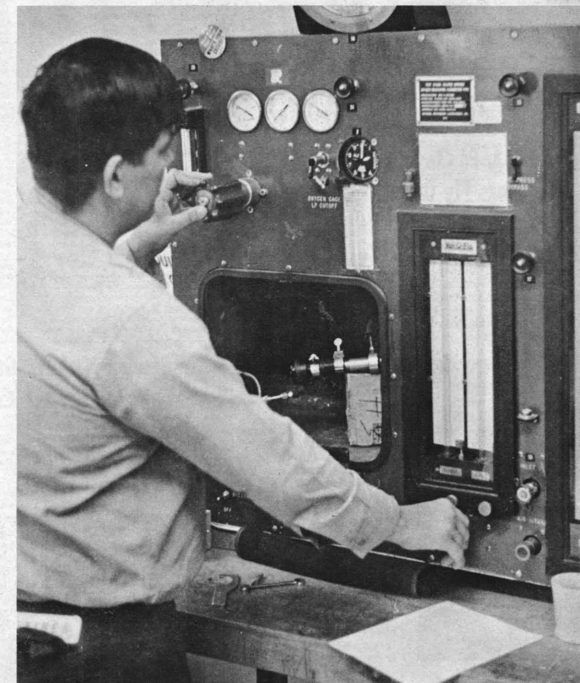
ABOVE — PR2 Robert Ruiz performs the daily maintenance necessary on the sewing machines used by the men in the Para Loft and Raft Shops to repair shrouds and raft equipment. BELOW — PR2 Don Gaines makes a check of oxygen mask regulator
