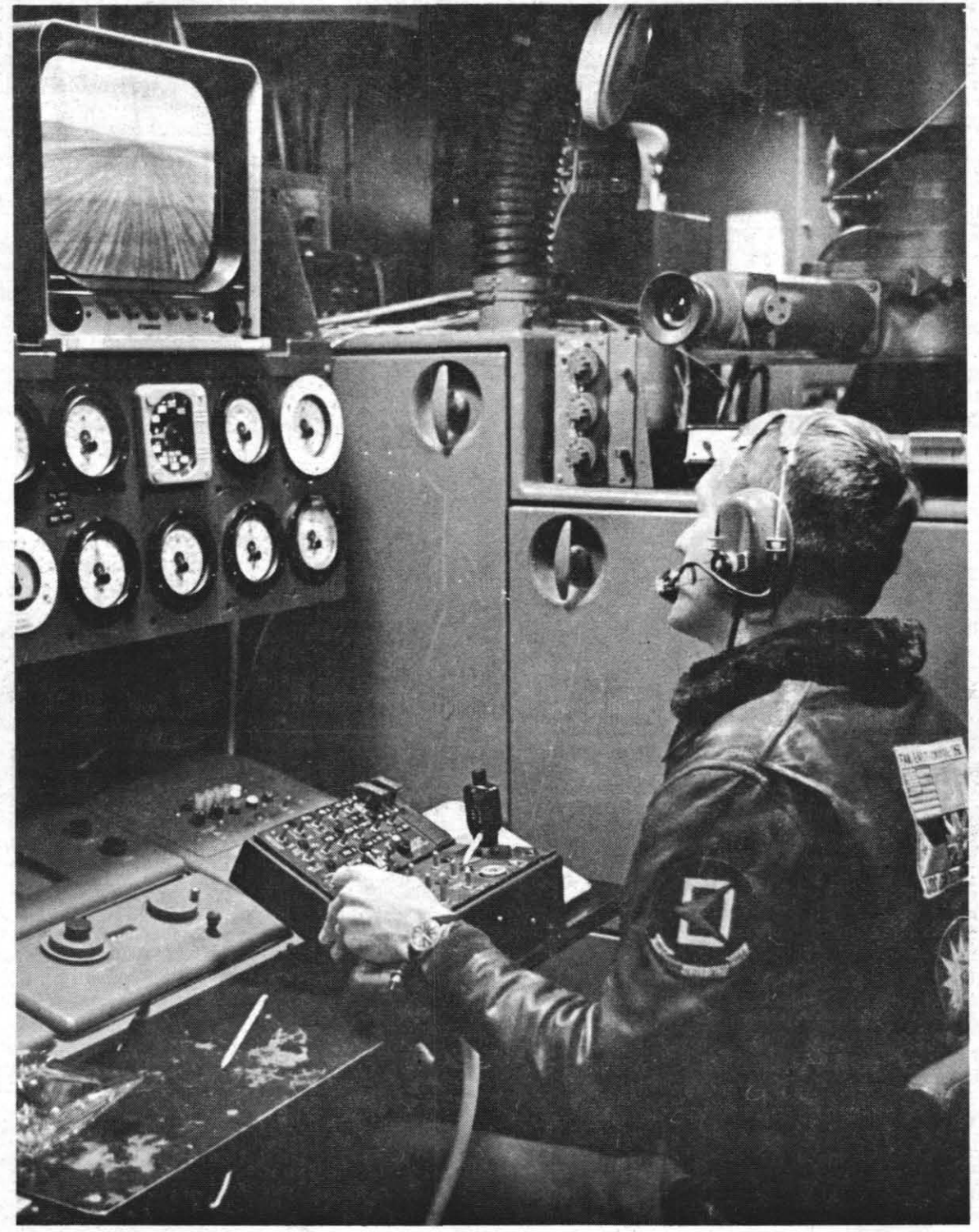
OUT-OF-SIGHT CONTROL —Lt. Virg Kempenaar of NAF is shown above at the controls of a target drone that has been modified to include a television camera in its nose. Flight controls in the drone are linked to this set-up (which is located in a trailer) and permits controllers to present the drone as a more realistic target device.
