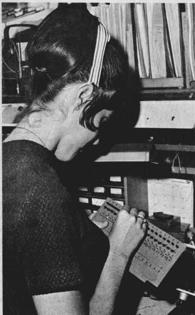
MATH MAJOR —Ann Allan, a Junior at UCLA where she is majoring in Mathematics, Physical Education and Psychology, is shown above installing components on a complex filter board for a doppler radar. Ann is working in the Systems Project Engineering Branch of AOD.
