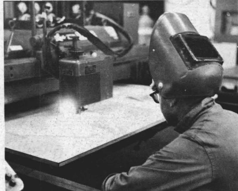
ABOVE—Henry Olinger is shown adjusting the controls of the Plasma Arc Cutting Machine as the torch burns through a 3-in. thick piece of aluminum. This Plasma cutting unit is mounted on a Linde Shape Cutting Machine, seen nearly surrounding Olinger. RIGHT—Olinger watches the Photocell Tracer Unit as it follows a line drawing mounted on a table. This unit follows any sketch, line drawing or outline rather than the costly templates of metal formerly used when the Douall Band Saw was used to cut non-ferrous metals. The unit is located in the southwest corner of the welding shop in Michelson Laboratory.
