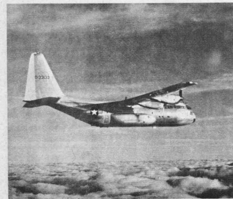
CLOUD SEEDER—Pictured above is an Air Force C-130 aircraft, which is the type used to "seed" clouds with Silver Iodide particles over droughted areas in the Philippines. The planes were based at Clark AFB.
