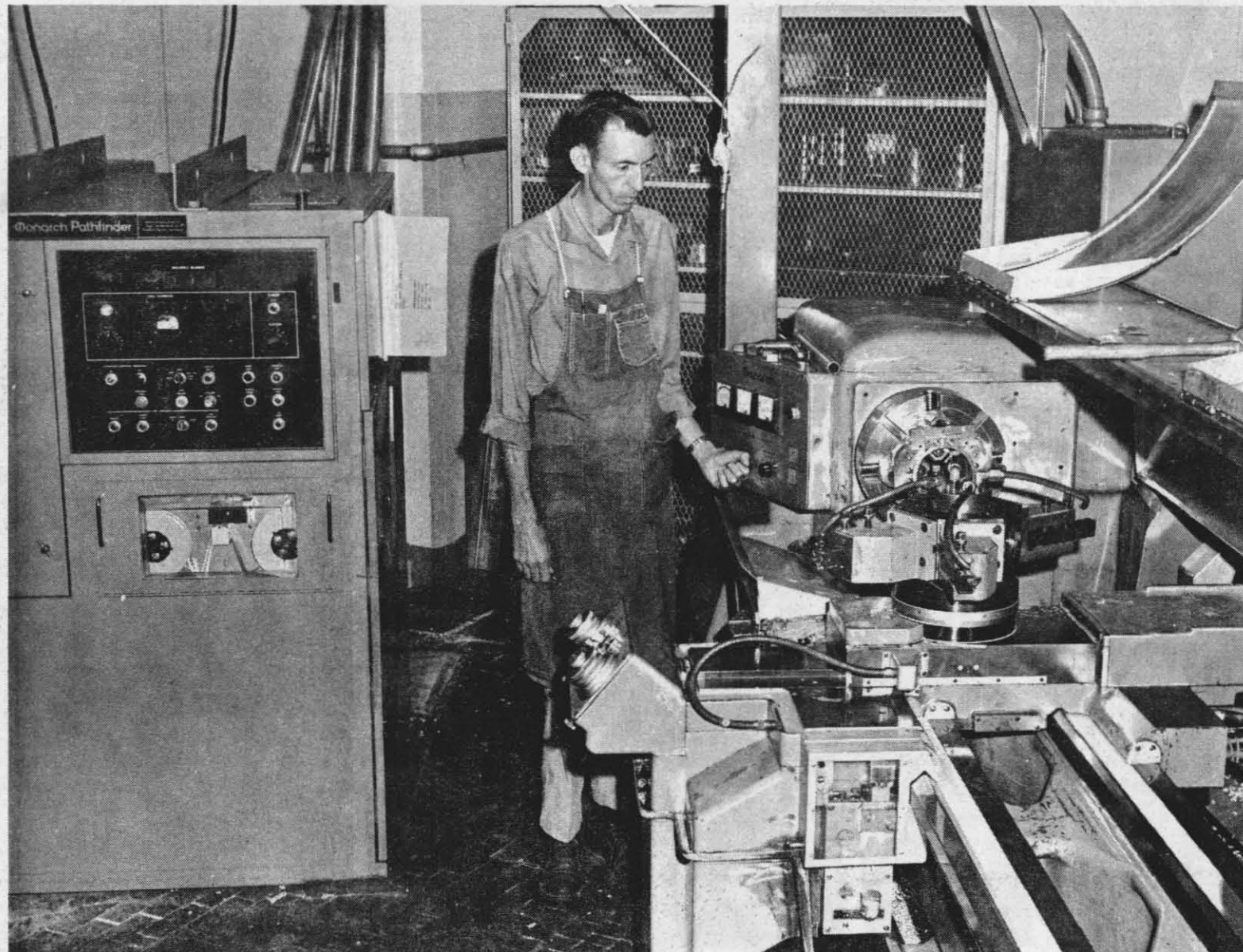
MONARCH LATHE — Jim Carter, Machine Model Maker, is shown above operating a Monarch Pathfinder full contouring lathe. The lathe turret has eight positions for tools which can be preset and indexed into position as called for by the
