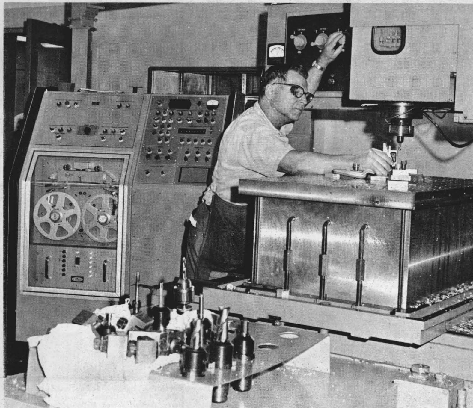
HEALD ACRACENTER —Bill Hobaugh, Model Maker, is shown operating one of the Heald AcraCenter Continuous Path Full Contouring Milling Machine. In the foreground are ad-
