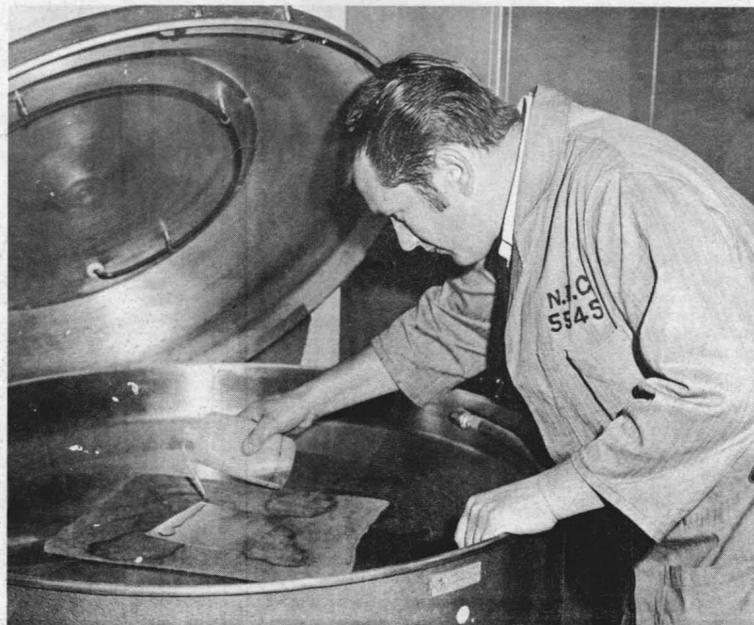
**ONE OF MANY TECHNIQUES**—Charles Knowles, Etched Circuit Maker, applies photo-sensitive emulsion to a board prior to spinning. Circuit card is spun at 120 R.P.M.
