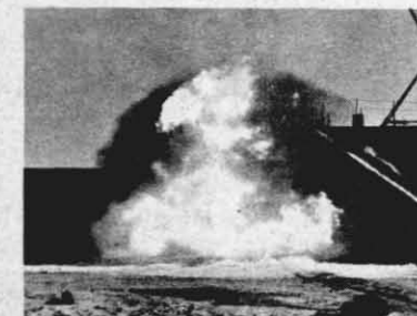
DETONATION —This series of photos was taken by a camera stationed outside the Firing Chamber. This type of data is also used to analyze detonation characteristics of explosions.
