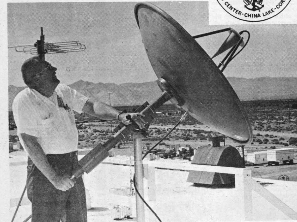
ANTENNA ADJUSTMENT —Carl Peters, Electronic technician, is shown adjusting an UHF telemetry receiving antenna on a new antenna platform located on the roof of Michelson Lab. The antenna is used to receive UHF telemetry signals from both ground and airborne vehicles at the Naval Weapons Center.
