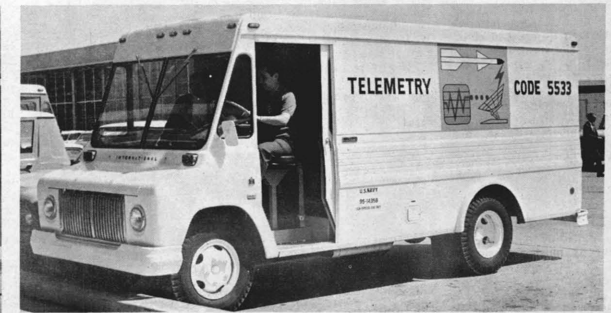
LOTS OF MOBILITY — Electronic Technicians Dan Childers (l) and George Barker get ready for a trip to NAF's "Hot Line" to perform telemetry preflight checks for a Sidewinder firing. The new mobile telemetry van will be able to receive transmit and record telemetry information and all UHF and VHF bands in remote locations.
