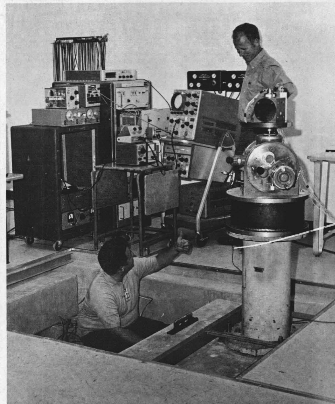
SHOCK ABSORPTION—Nick Schneider, Associate Head of the Guidance and Control Division, adjusts the air pressure to the pneumatic isolation pads on signal from Al Herbert, Code 40 Electronic Technician. Each test table in the new lab is individually mounted on concrete pads weighing
