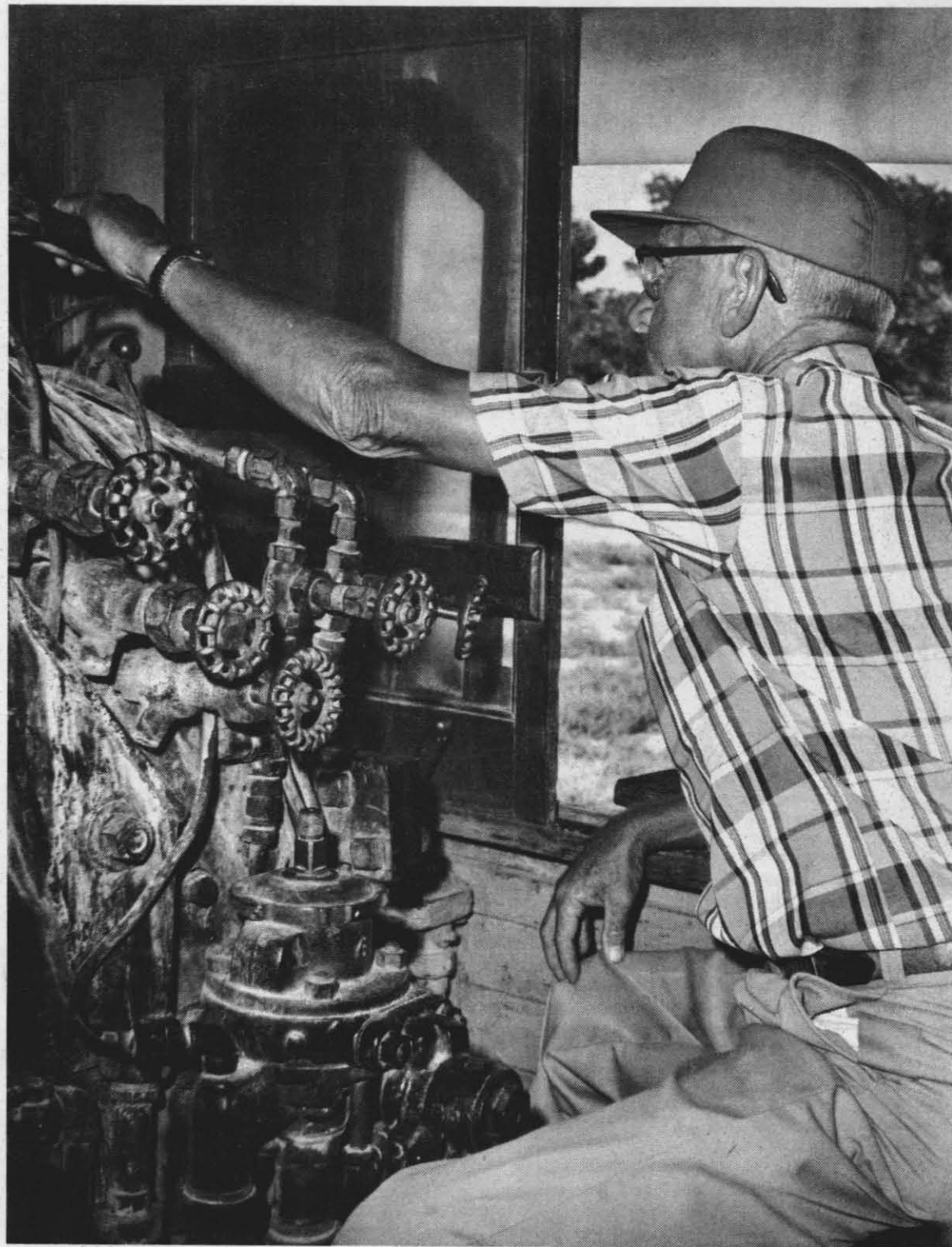
FRANK ROUSH advances throttle of the Slim Princess locomotive, "Old No. 9", to show how controls are handled. Roush, a former railroad man, tells Museum visitors
