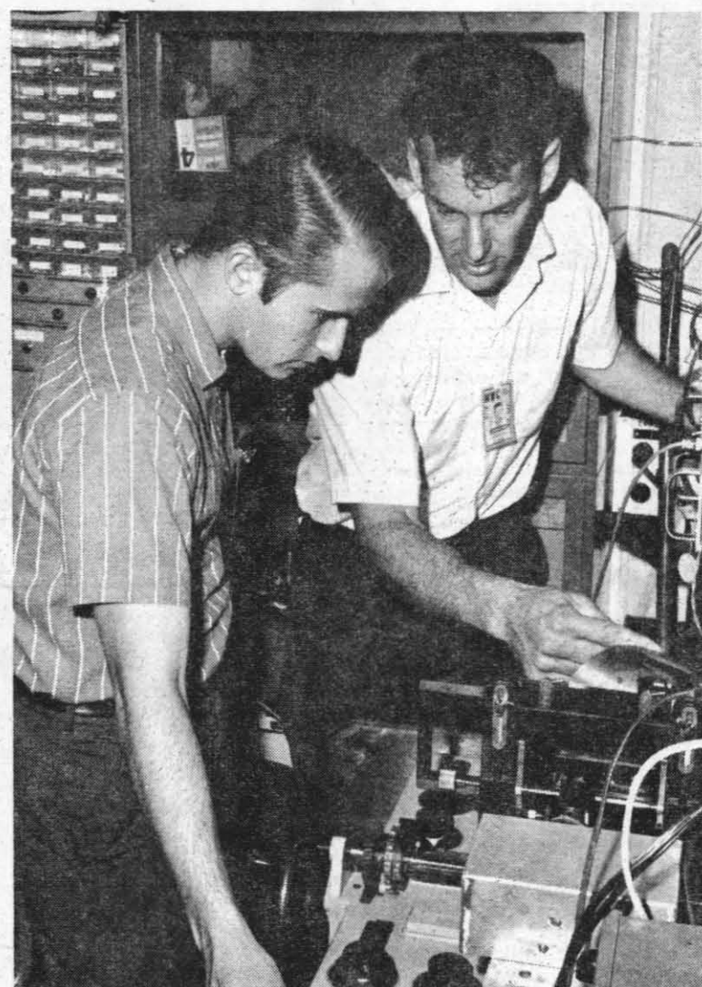
PHYSICAL OPTICS — John Pearson (l) is shown being taught the finer points of using a densitometer in the Research Department. Richard Roberts explains the operation of the machine.
