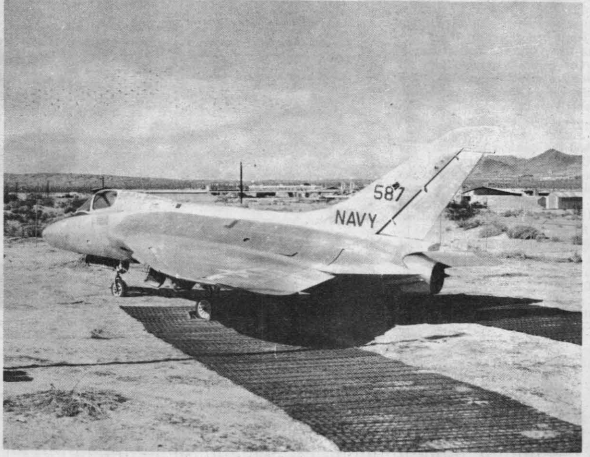
RETIRE CHAMP — The Douglas XF4D-1, above, one of two such aircraft made, at one time held two world speed records and was the original test bed for the famous GE J79 engine. The Center has other aircraft of historical value in its inventory.
