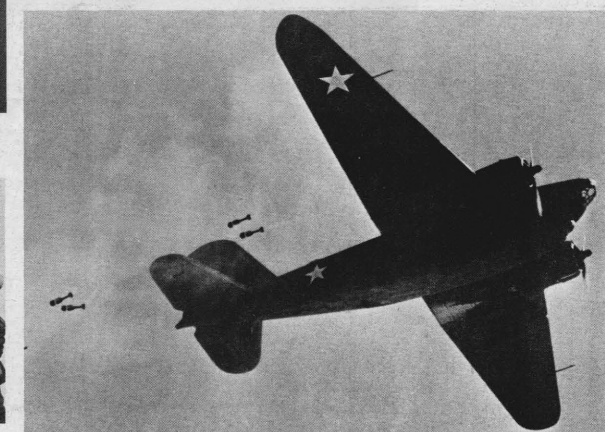
EARLY RETRO ROCKETS — It is reported these retro rockets, before the forward firing rocket, were being tested at Salton Sea in 1942 as a defense against submarines.
