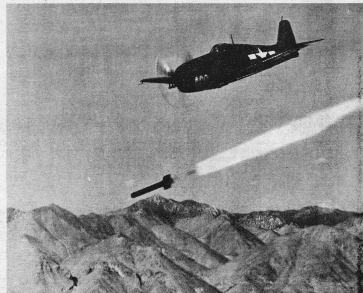
TINY TIM — An 11.75-inch torpedo-shaped rocket, developed during World War II, is fired over China Lake ranges during 1944. Operations were conducted from Harvey Field before the air units moved to Armitage Field. Tiny Tim weighed 1,250-lbs.
