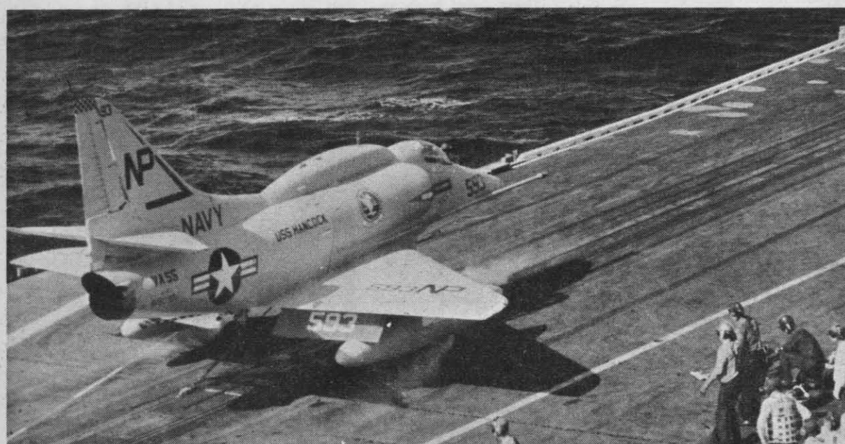
A DOUGLAS A-4 SKYHAWK—Smallest combatant striking jet aboard the Hancock awaits the order to launch. Hancock was the first US Navy carrier to install steam catapults. With these catapults, the optical landing system and an angled deck, Hancock is capable of operating the most advanced naval aircraft in service today.
