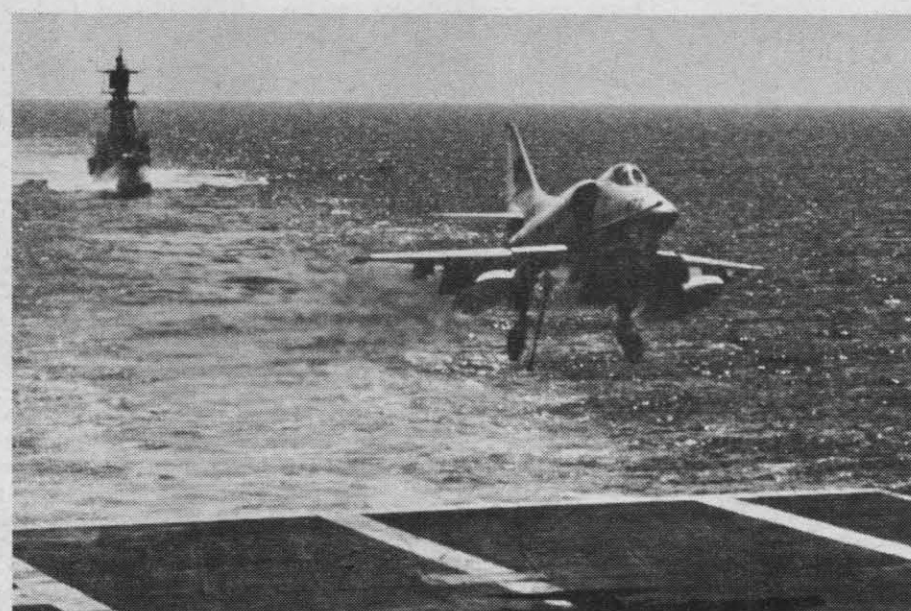
A BIRD COMES HOME—This A-4 Skyhawk, single-seated attack jet, approaches the Hancock's flight deck for a landing. In this routine maneuver, the plane's landing hook engages one of the steel cables shown in the foreground and stops the plane.
