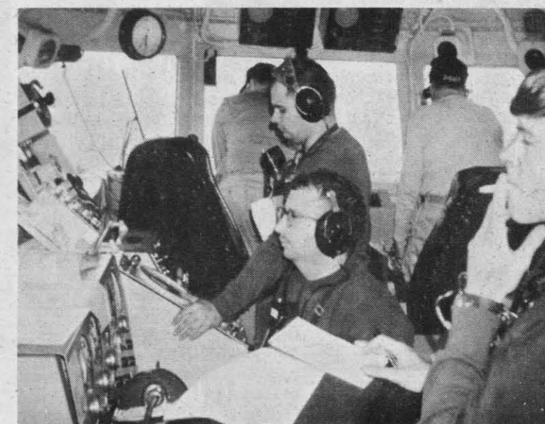
HIGH ABOVE THE FLIGHT DECK this "Pri-Fly" unit organizes the sequence and monitors the carrier's plane flights. Compact and complete with all forms of communication gear, the unit is equivalent to the control tower of an airfield.
