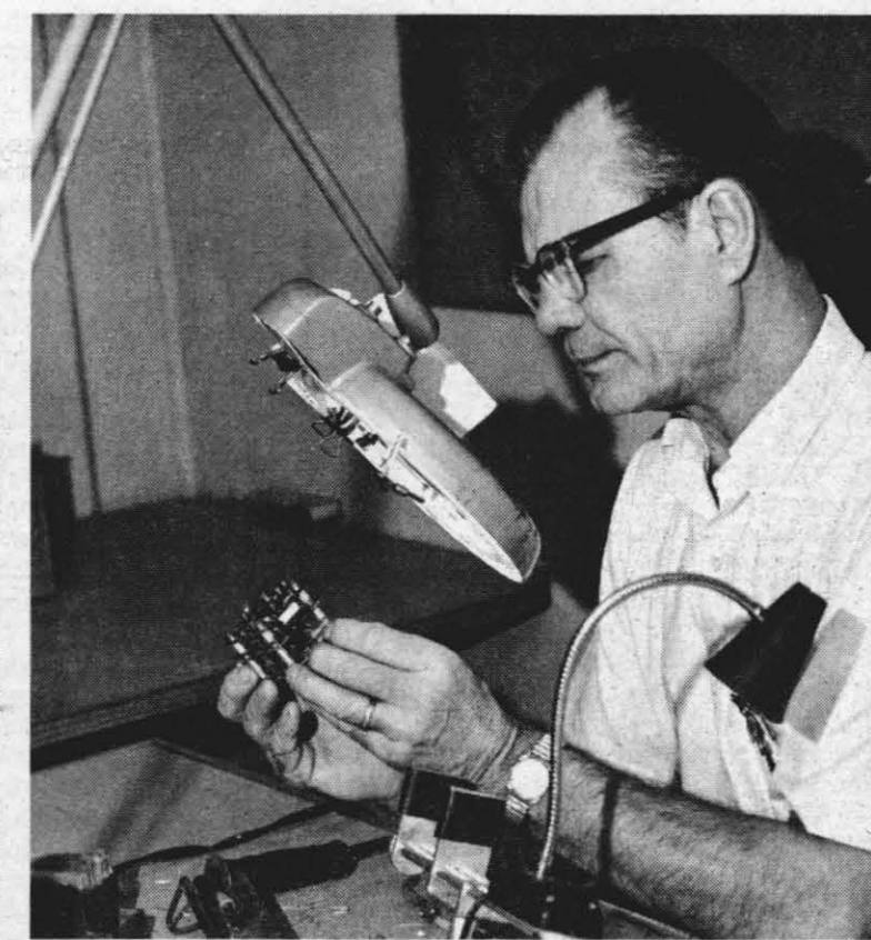
PROFESSIONAL AT WORK — Building models is one way of passing time for some people, but for Elwood S. Neuman of the NWC Corona Laboratories Electronic Hobby Shop, it takes an electronics technician's know-how to assemble "stacks" including its complete circuit for use in a missile.
