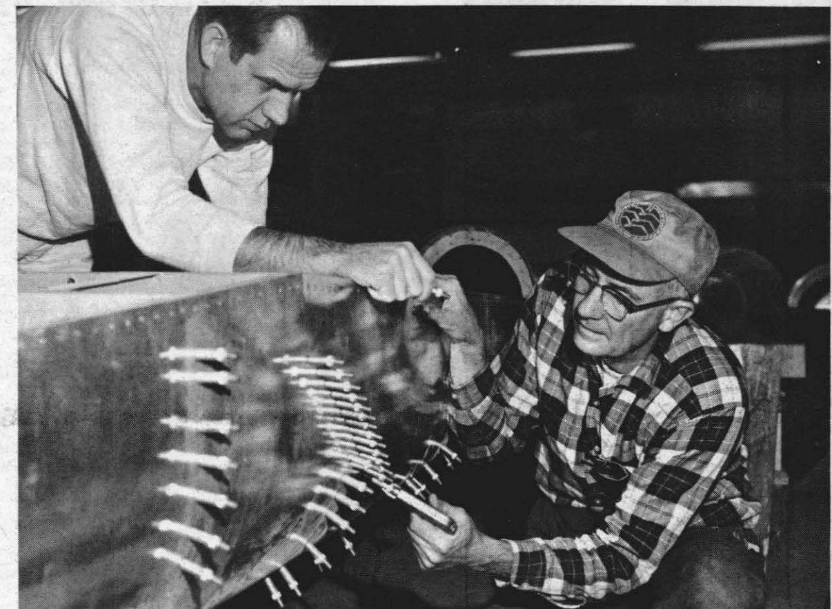
BUILDING FOR LIGHTNESS — Charles Drew installs "cleco fasteners" through skin of fuselage, holding seat in place. Later, rivets will be installed. Helping him is new club member Jim Gladney of Associated Aero Science, learning from ground up.
