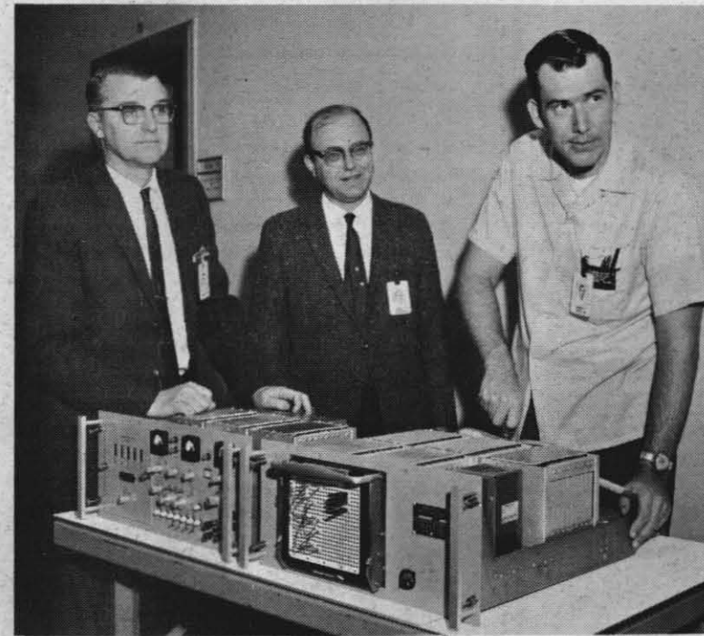
FIRST SERVICE TEST MODEL — T. B. Jackson (left), Head, E. D. Herberling, Associate Head, Instrumentation Division, and R. D. Sweet, Electronics Technician, shown with the first service-test model of the PAM telemetry decommutation system. The units are being transferred to Naval Weapons Center China Lake to establish initial capability for processing the PAM/FM data. The PAM telemetry decommutation was designed and built at NWC Corona Labs.
