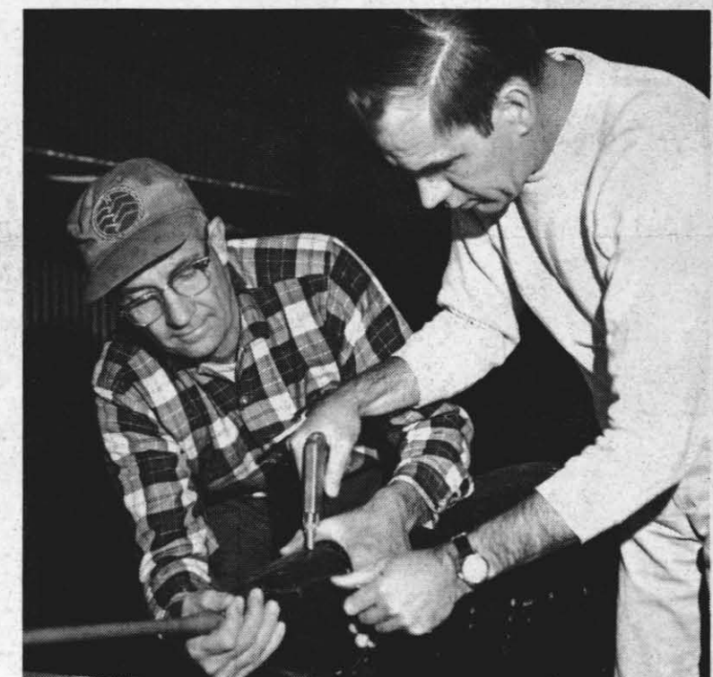
ATTENTION TO DETAIL — Drew and Gladney check nose piece of soaring craft for perfect alignment as Gladney fastens another rivet in place.
