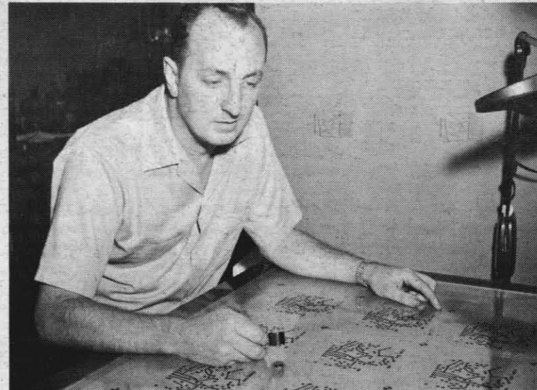
AWARD WINNER — Harold G. Watson demonstrates the accuracy of his winning beneficial suggestion on a light table. A master grid of solid, distinct black lines on a transparent mylar film allows positioning of printed circuit drawings to within 0.005-inch tolerances.
