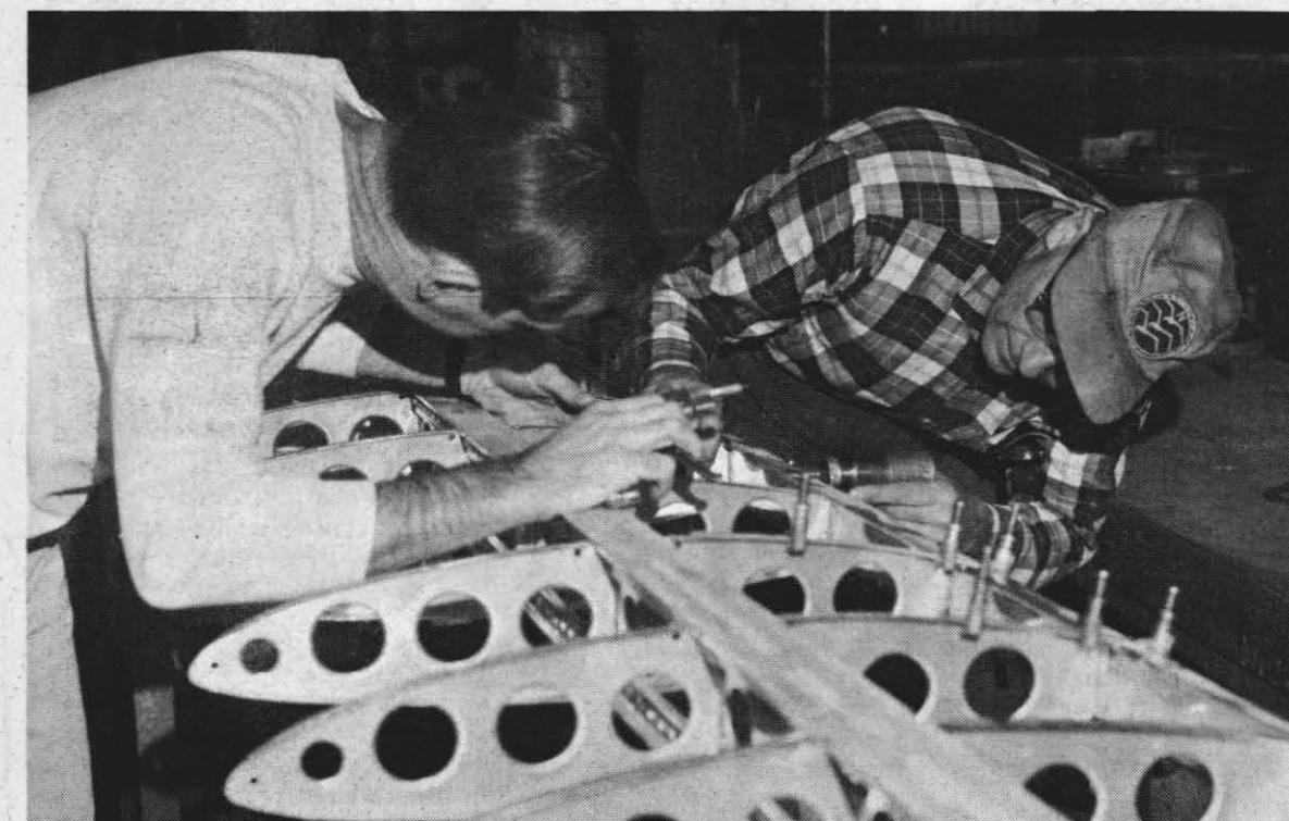
BUILDING THE WING — As Jim Gladney holds rib steady, Charles Drew installs cleco fastener through "drag strut" along trailing edge of wing. Fasteners projecting upward along ribs in foreground hold thin alignment strips in place.
