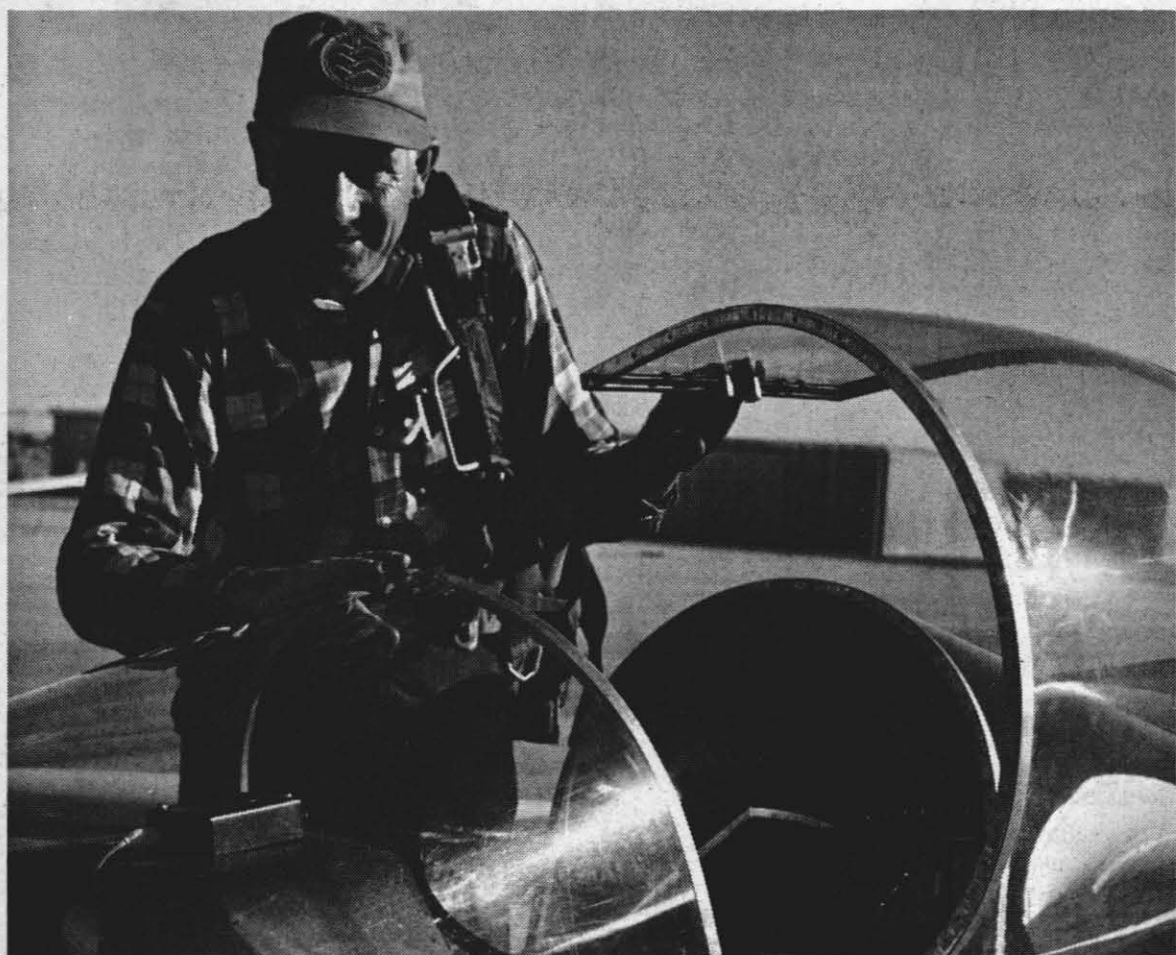
READY TO SOAR — Charles Drew prepares to board his Schroeder HP 11-A craft at Inyokern Airport, "one of the best," according to Drew. Small box atop instrument panel is audio variometer, whose chirping noise varies with altitude.
