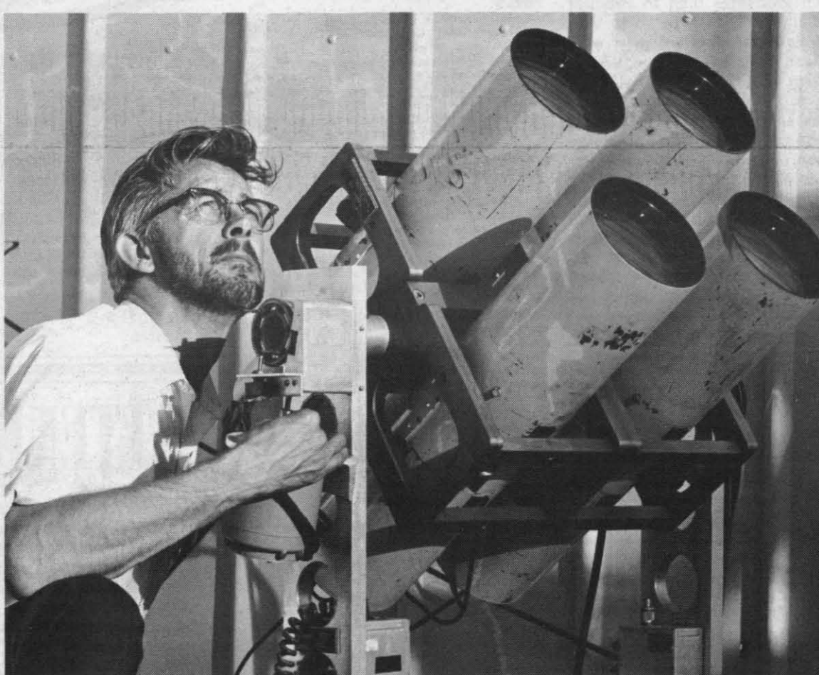
MEASURING AIRGLOW — Jim Moore of Earth and Planetary Sciences Div. orients telescope battery toward the patch of sky furnishing him and his colleagues with new information about the ionosphere. The 'scopes catch faint "airglow" from the ionosphere on clear, moonless nights, which is then registered by photomultipliers and recorded on magnetic tape for analysis. Airglow is from breakup of ions after intense sunlight radiation ceases at night. The ATS-1 is being used. —Photo by Jerry Willey
