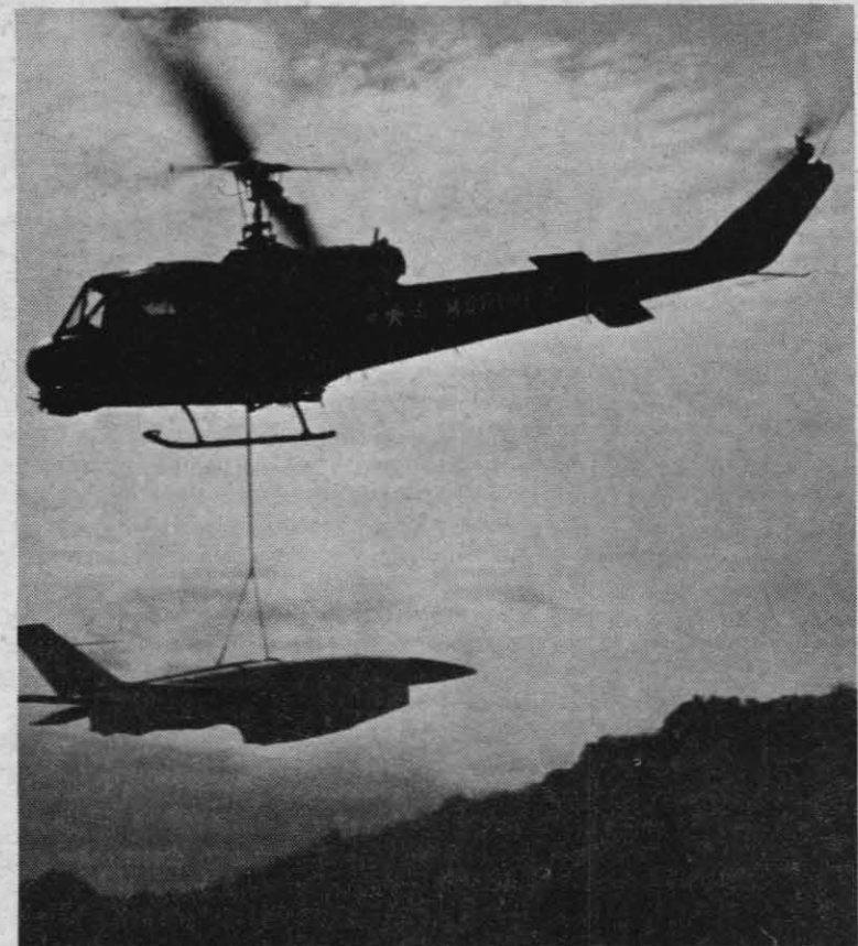
ONE HEAVY LOAD —Capt. Overfield and his UH-1 helicopter lift the 2,000 pound Firebee drone from its precarious resting place on the edge of a cliff 6,500 feet high. Only the Captain's skill and knowledge of the aircraft made the mission possible. —Photos by Lt. Pete Ferrentino
