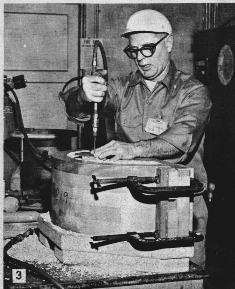
OUTER CORE WITH CO-2 SODIUM SILICATE
