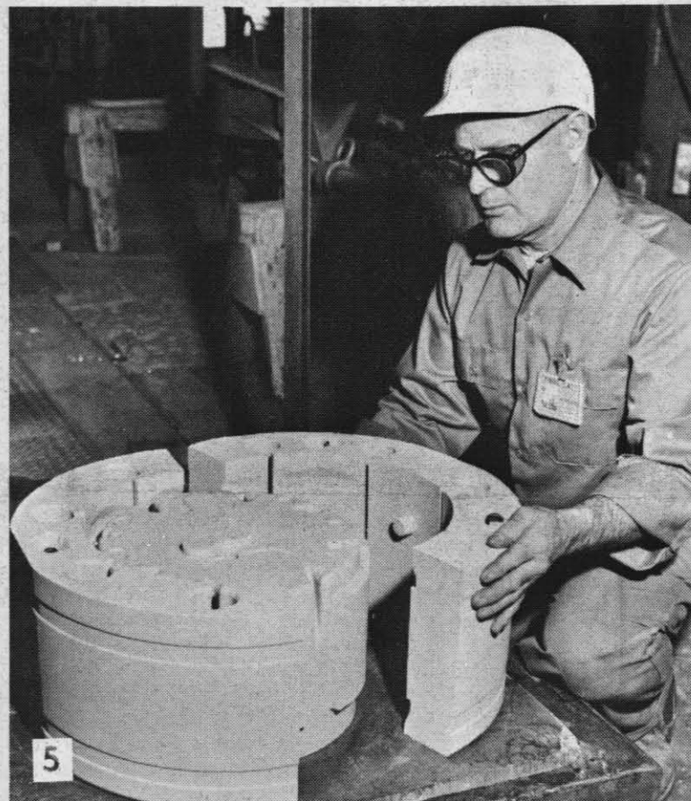
ASSEMBLING INNER AND OUTER CORES
