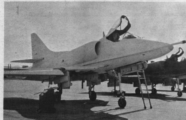
NOW YOU SEE IT, NOW YOU DON'T — Or at least, not when it's flying. ABOVE, VX-5 men (l-r) AMH3 E. Smith and AMS1 E. S. Pujol spray light sky blue paint on A-4 aircraft, while project officer Lt. Pat Nicolls judges effect. BELOW, finished plane tries to blend in with sky. It proved hard to find as it flew over "B" Range cameras in tests.
