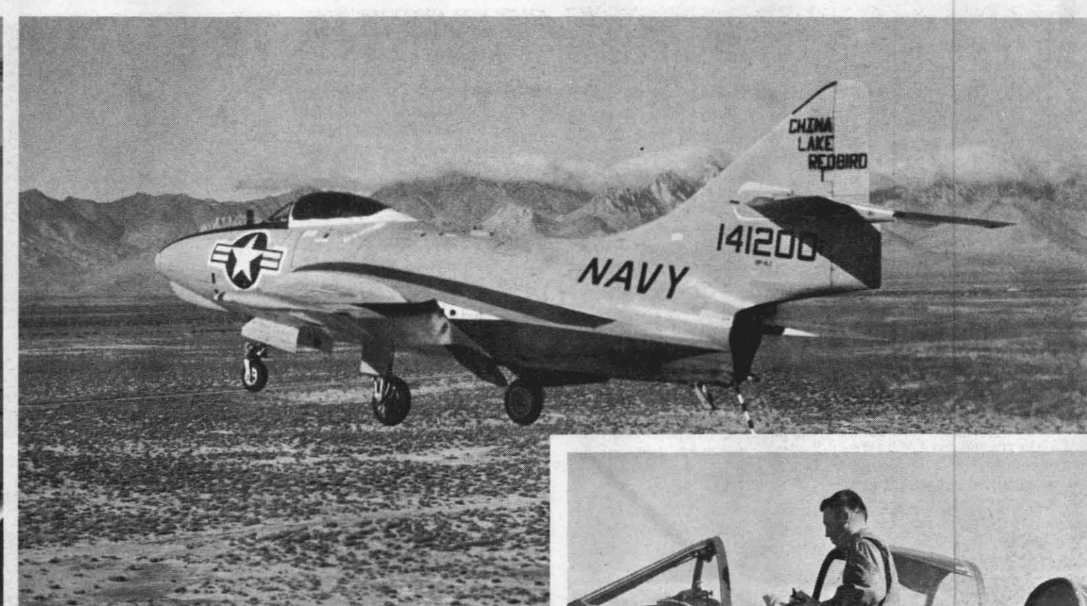
A STRANGE PAIR — Strange as it may seem, the aircraft at the right and the one above will work as a team. Lt. G. L. Gottschalk, NAF pilot, gets ready to board a T-28 propeller driven, two place aircraft. From this T-28, the pilot will control the F-9 target plane (above) through part of its mission. This picture, taken from the back seat of the T-28, gives a good idea of the small distance between aircraft. Note that the canopy on the F-9 is painted black. There is no pilot.
