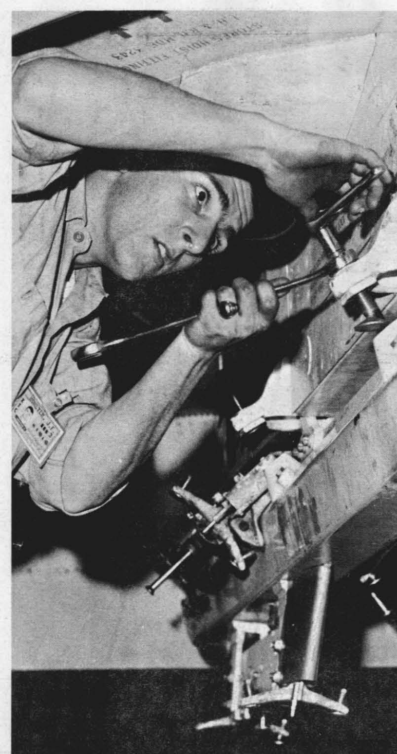
BOMB RACK —VX-5's J. Homeyer, an Ordnance Airman, tightens the lugs on TER bomb rack of F-4B. Men like Homeyer are highly skilled in their work.
