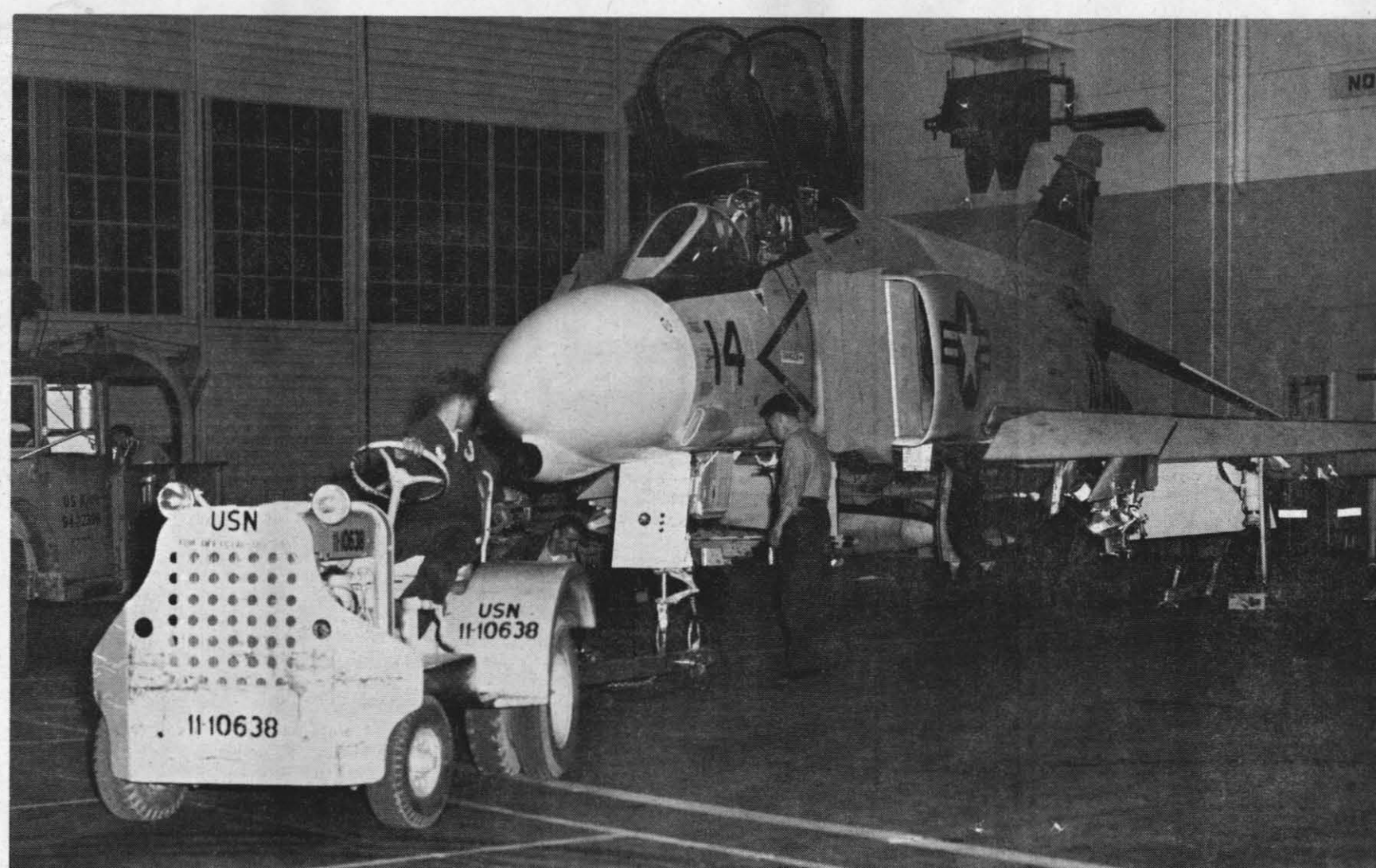
BURNING MIDNIGHT OIL —The night check line crew at VX-5 makes preparations to tow a F-4B out of the hangar for an engine turn-up. This is but one of the many maintenance jobs performed by the Squadron crews.
