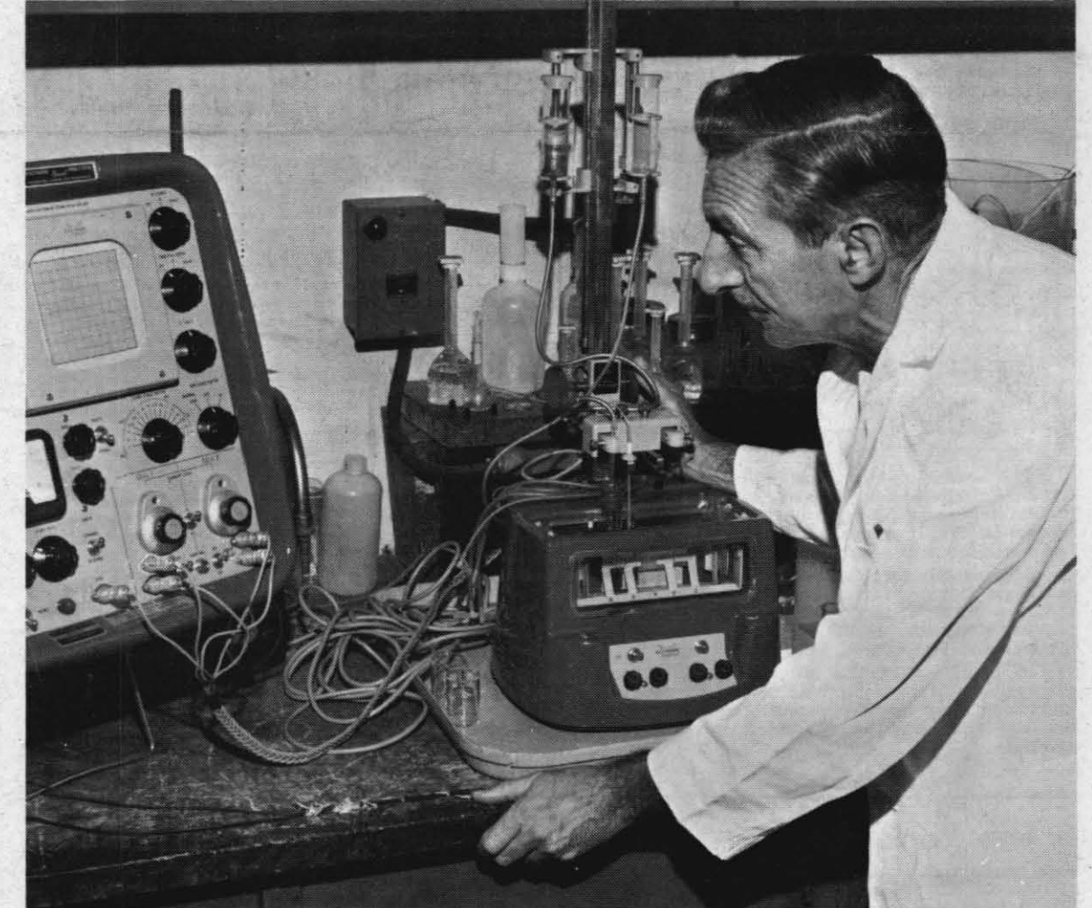
WATCHING FOR EVIDENCE — Jerry Whitnack, head of Code 50's Electrochemistry Lab, eyeballs cathode ray screen (left) for evidences of trace elements in water sam-
