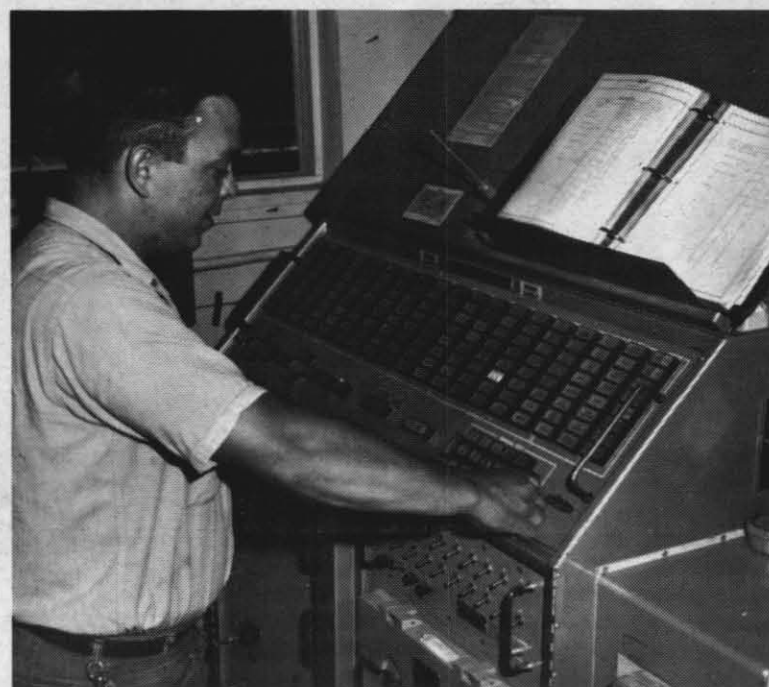
TESTS, TESTS AND MORE TESTS — ATN2 John H. Klomfas runs through the Firebee "check out" list prior to its acceptance for the test. This is by no means a simple operation. There are over 60 pages in the "check out" list that require 560 individual equipment checks.
