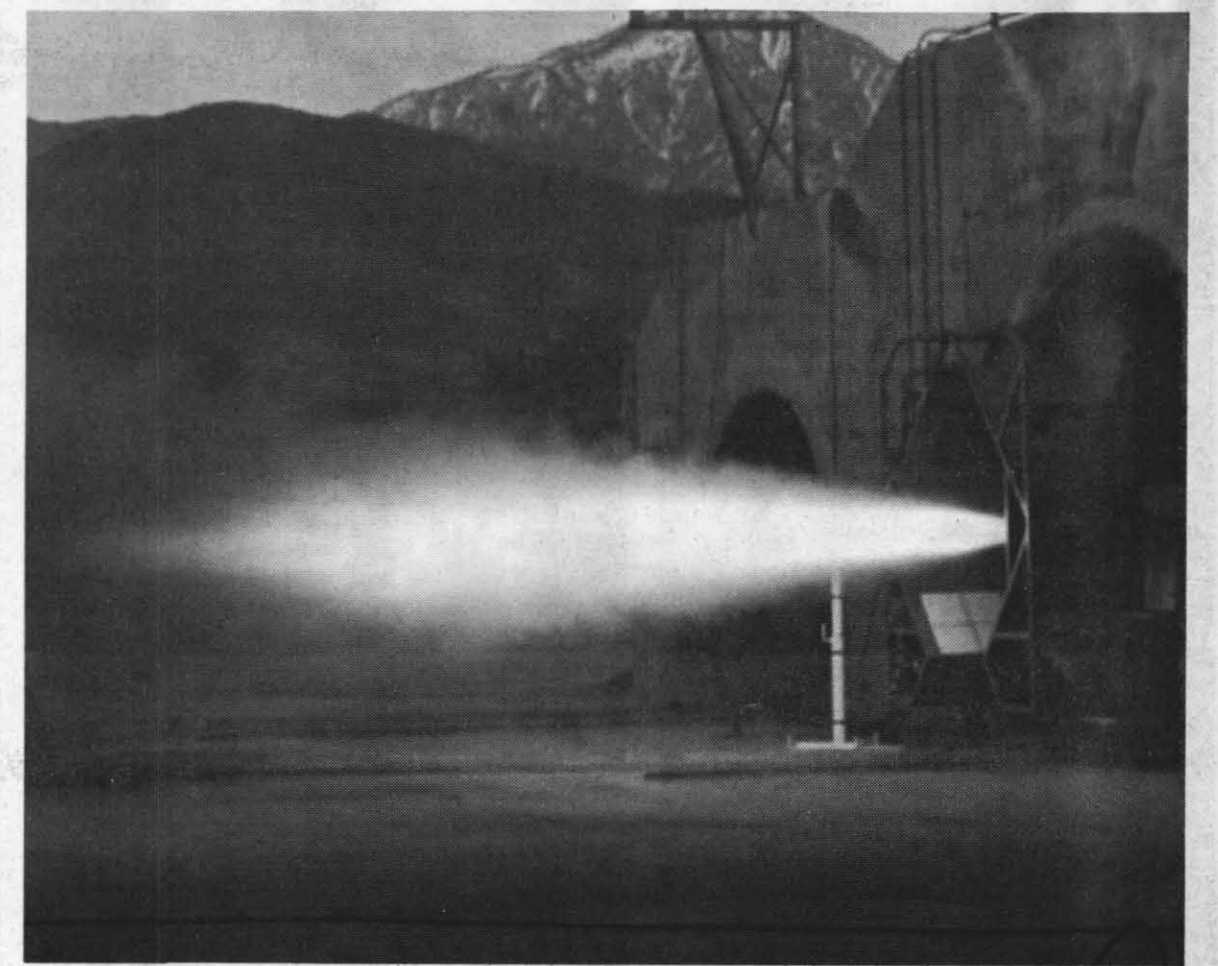
PULSE FIRING —Five-pulse solid propellant rocket motor fires successfully at Lockheed Propulsion Company's Redlands, Calif., proving ground in test conducted for NOTS. The energy controlled motor was developed to demonstrate feasibility of pulsed rockets for use in an air-launched Navy weapons
