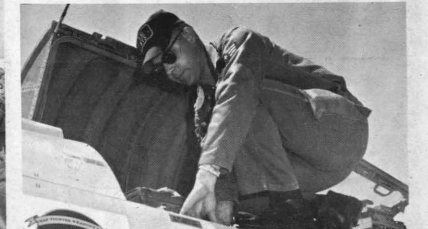
ANTENNA CHECK—A very important piece of equipment in any aircraft is its radio. Here the UHF antenna is being inspected. Each crew member is capable of handling several different functions of the check out.
