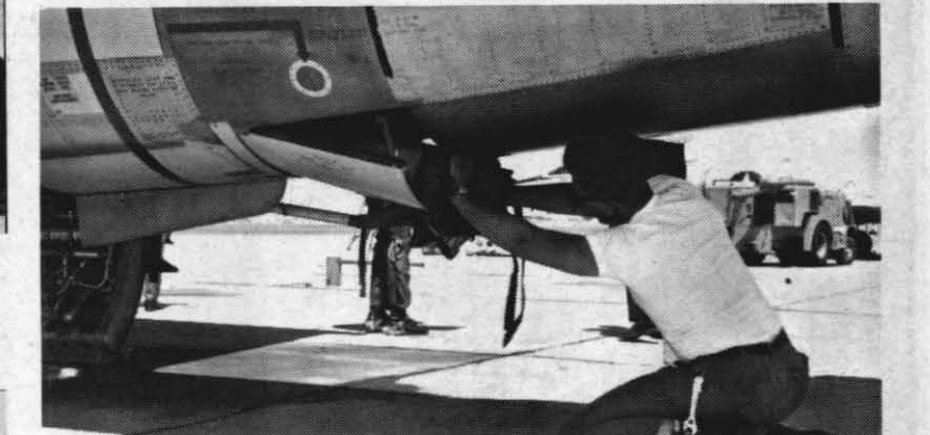
WHOA —When you're making a final approach at 170 mph, and the runway looks a little short, this "second set of brakes" comes in mighty handy. Here you see the drag chute being installed by one of the crewmen. It takes about a half hour to re-pack the chute after landing.
