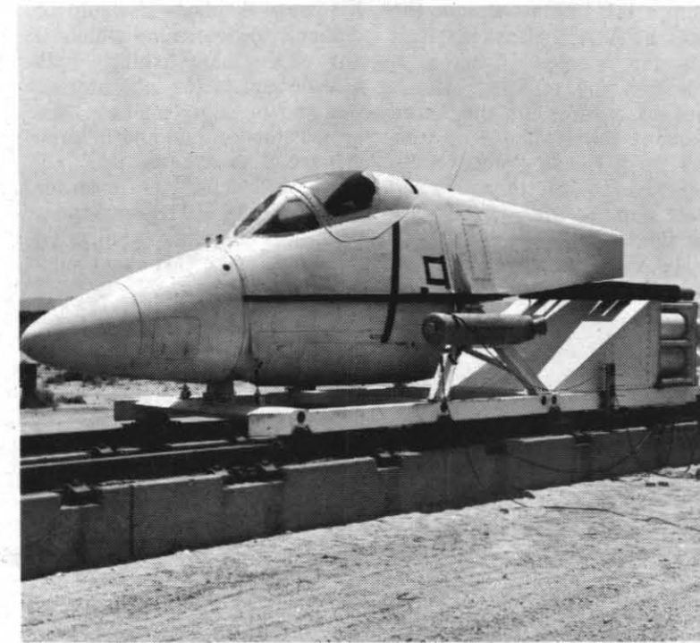
SPECTACULAR DEMONSTRATION —Without a doubt, the most spectacular and impressive actual demonstration was the firing of SNORT, a tracked vehicle designed to test the ejection seat. It has saved many lives.
