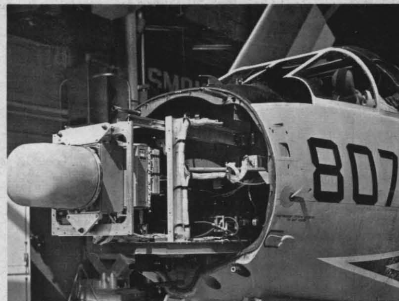
MICROMINIATURIZATION — The airborne XR-45 Multi-mode radar is shown installed in nose of former F3D light attack fighter. It's first such system with micro circuitry.
