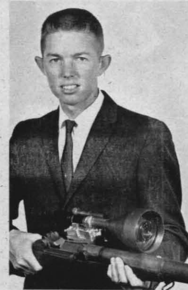
SNIPERSCOPE — A laser rangefinding sniperscope is nearly completed by Ted Bergman, physicist with Photophysics Br. of Code 30, after nearly two years effort. The new "eye" uses superconcentrated light and adds only 4 pounds to the rifle.
