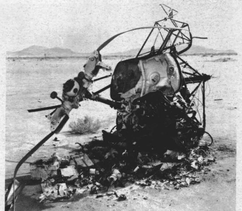
AFTER HIT BY REDEYE —Remains of drone H-3 helicopter, hit by Redeye missile. Other drones used in development and evaluation included Q2C and F-9 jets, KD2R prop drones and, in early phases, thermal devices on tethered balloons.
