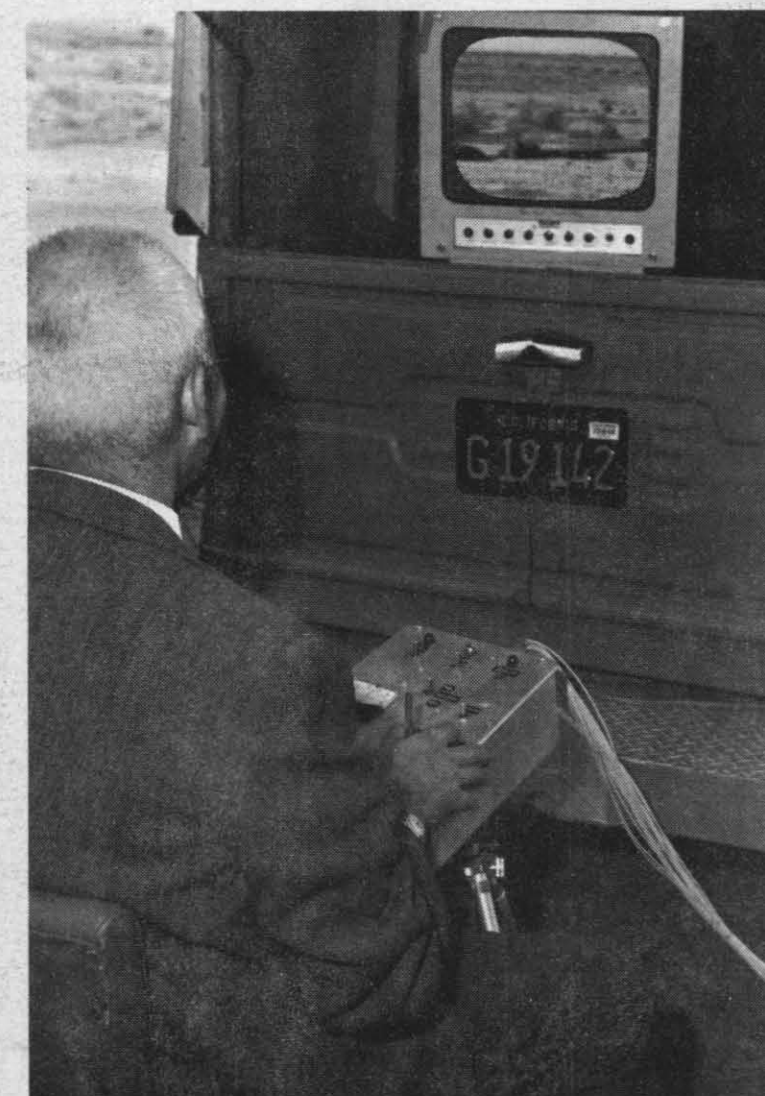
WHAT FIREBEEBLE SEES through its fixed lens is pictured on monitor screen for benefit of operator-builder Lee Dinapoli at his control console.
