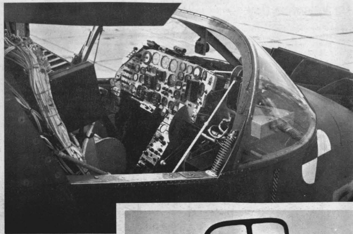
TANDEM COCKPIT OF XV-5A. View shows open louvers of nose fan, used in vertical flight and hovering. Craft flew in from Edwards AFB, refueled at NAF between tests on golf course driving range.
