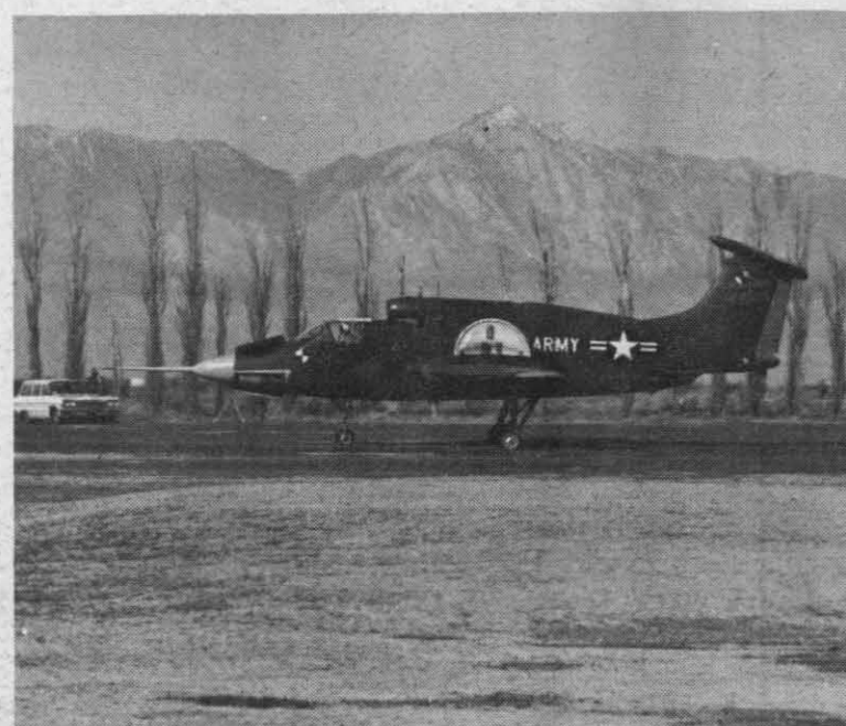
RISING FROM TURF of NOTS golf course driving range, XV-5A shows capabilities in rugged or unprepared terrain. Effect of downblast from fans in wings and nose was here measured against that of H-21 helicopter. Site was provided with typical Army command post tents for the tests.
