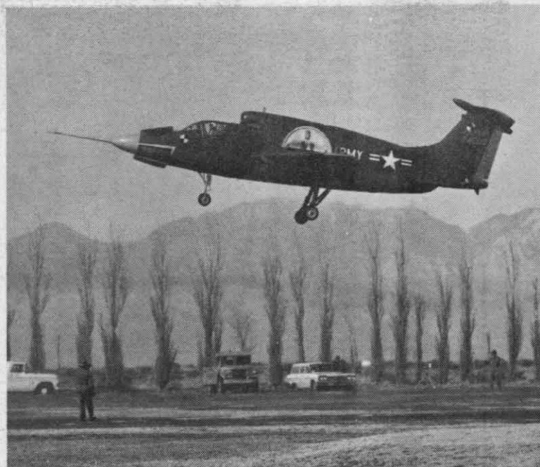
WING FAN OF XV-5A is checked out at NAF. One in each wing and one in nose, fans are free-rotating, powered by deflected jet exhaust. Semicircular vanes close as craft converts to horizontal flight.
