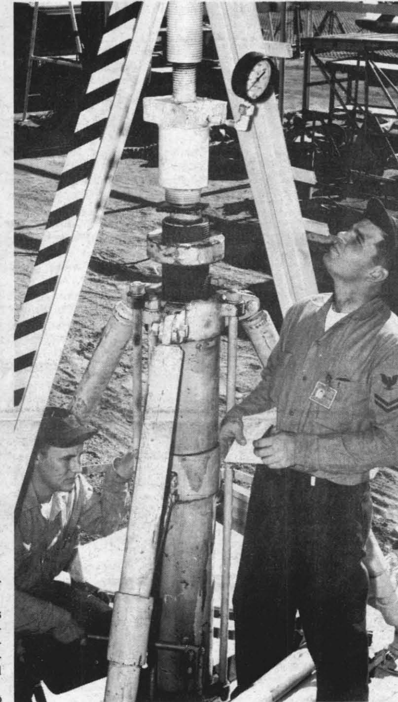
TESTER CHECKS OUT —Floyd Goldy, AMS-2, pumps pressure into 25-ton wing jack being tested in jack tester, while Auren Frei, ADJ-2, takes readings from gauge. The pair designed and built device to fill need for convenience, economy and speed at NAF. Tester stands seven feet tall, is eight feet wide and weighs two and a half tons.
