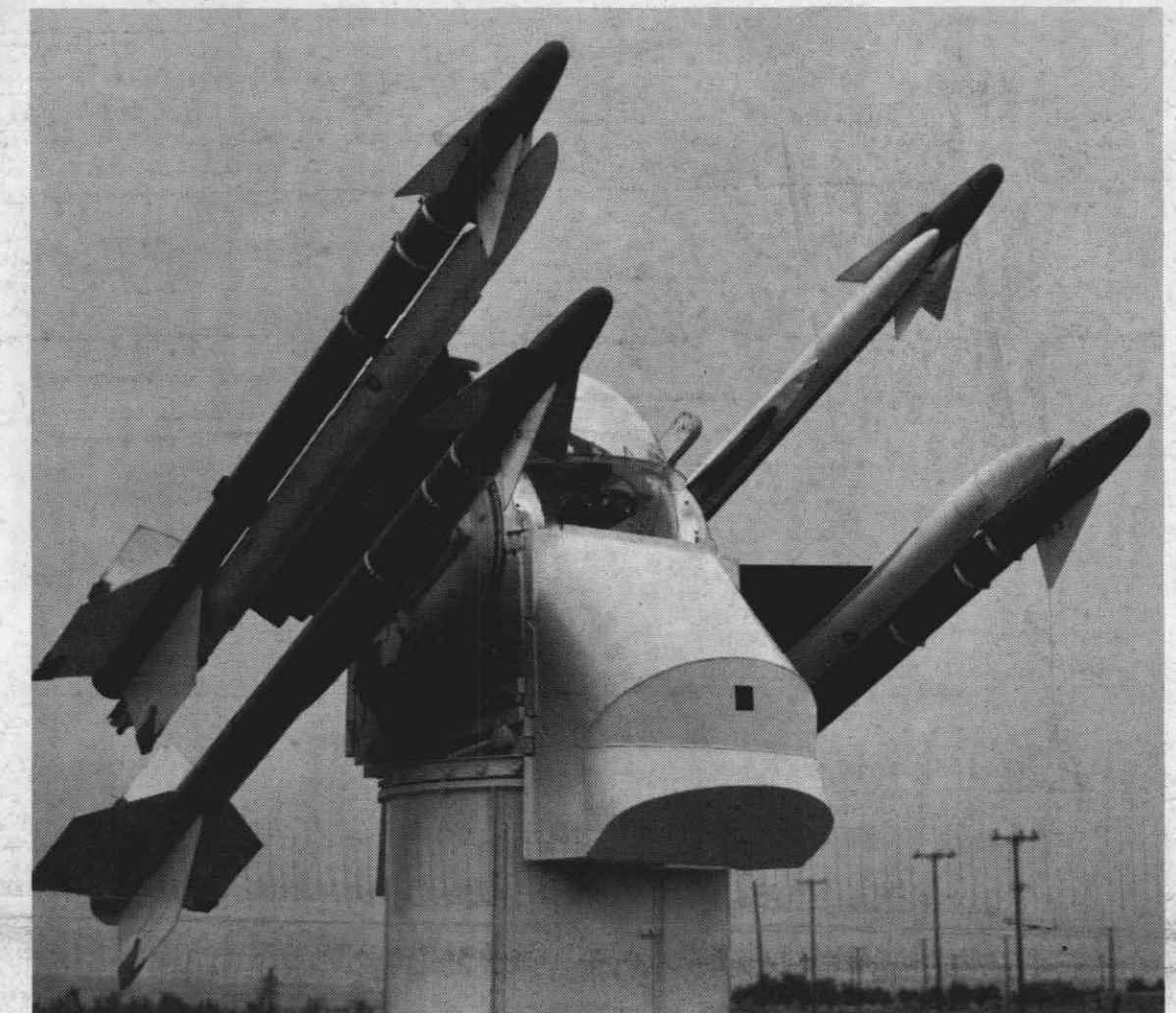
CHAPARRAL HAS LETHAL STING of four deadly Sidewinders. System is being developed here for the Army to provide its forward-area troops with an air defense from low-level aircraft attack. System will be mounted on Army XM548 tracked vehicle.
