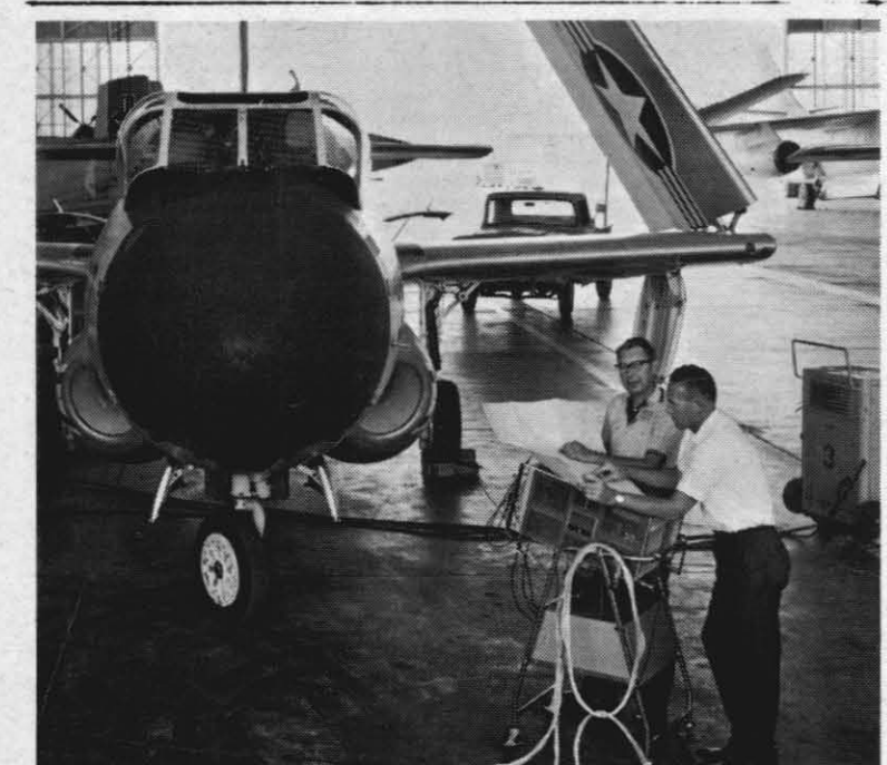
TECHNICIANS REVIEW PROSPECTS of XR-45 radar installed in nose of TF10B jet. Alfred B. Ferris (left), asst. project engineer from AOD, discusses nation's first micro-miniaturized airborne radar with Autonetics technician.
