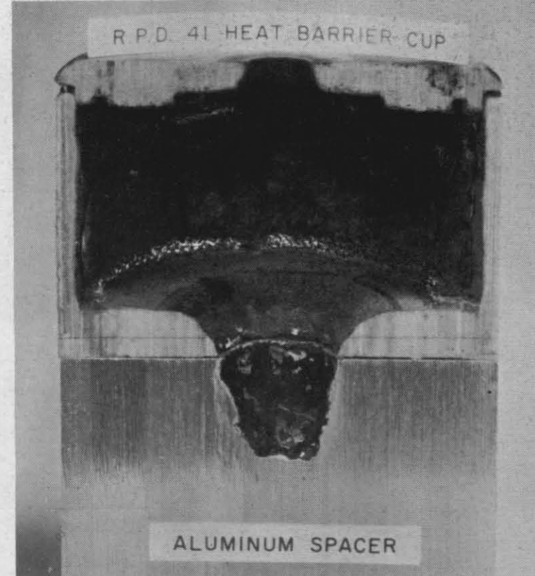
WITHIN FIVE SECONDS, "vortex effect" created by 250 revs per second of BOMROC sustainer motor test segment, caused burning propellant to drill through heat barrier and aluminum spacer. Propulsion Dept. team solved impasse with "diffuser" of graphite that gathers gases from circumference.
