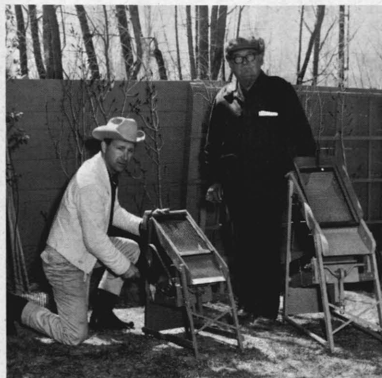
DRY WASHER DEMONSTRATION—Ken Miller of Central Staff demonstrates to "Pop" Lofinck one of three placer gold dry washers which he has developed.
