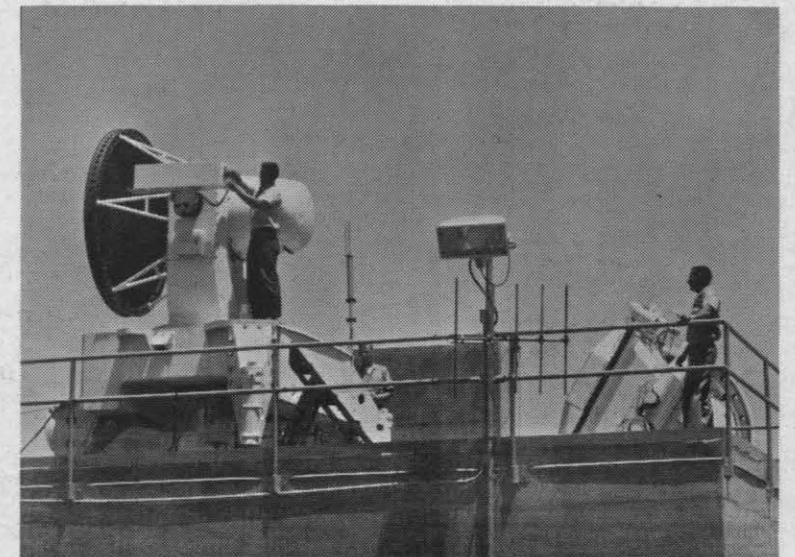
ATOP GUIDANCE RADAR BLDG., Richard Eakle, FTM-3, aligns TV camera (left, with horiz. white box) with the modified TTR-1 radar. Chief Richard Benbow (r) supervises work. Navymen operate facility, assist development.
