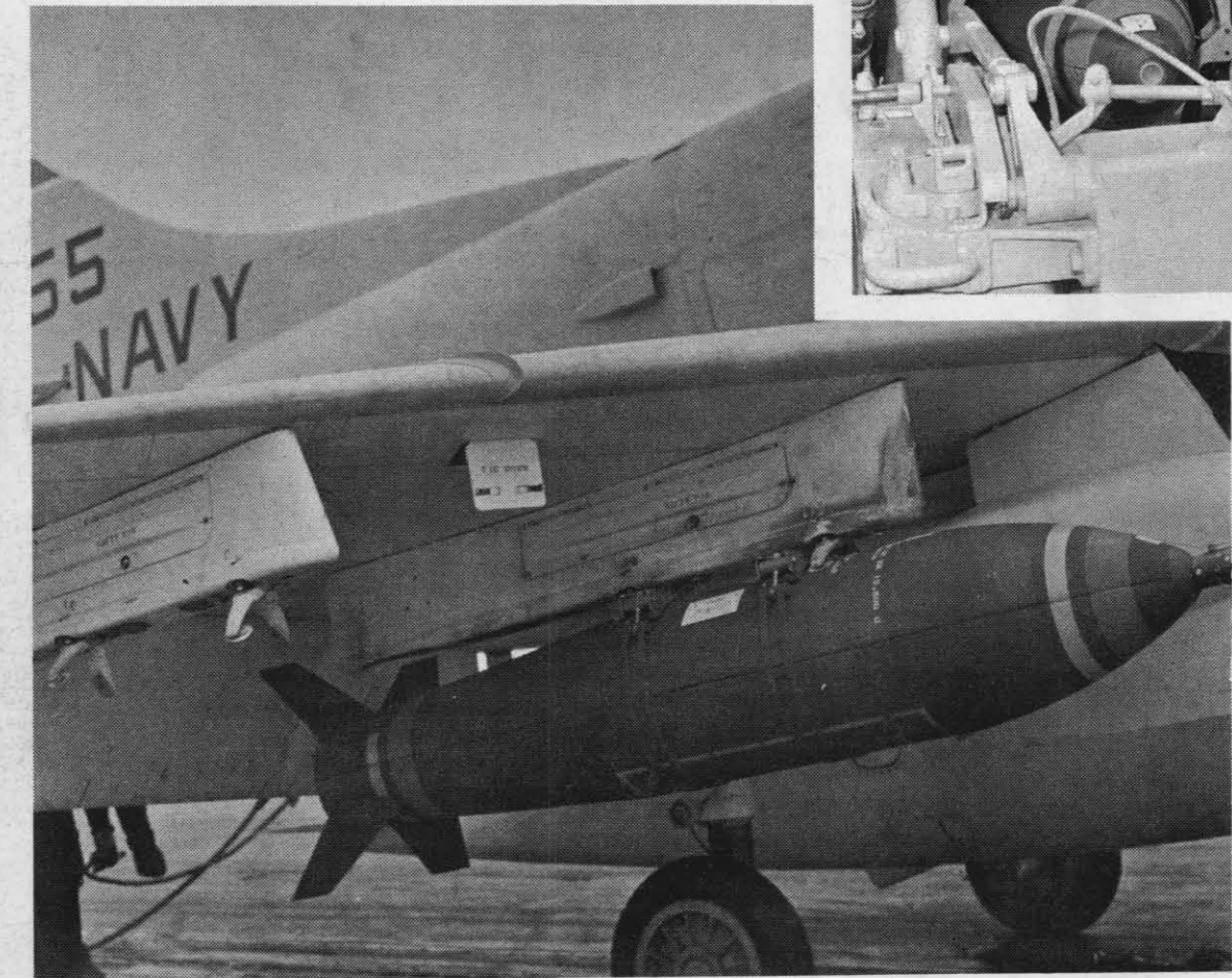
SCOTT BURNS , aviation ordnanceman, (above), loads SADEYE on inboard station of an A-4 Skyhawk during deployment aboard the Kitty Hawk.
