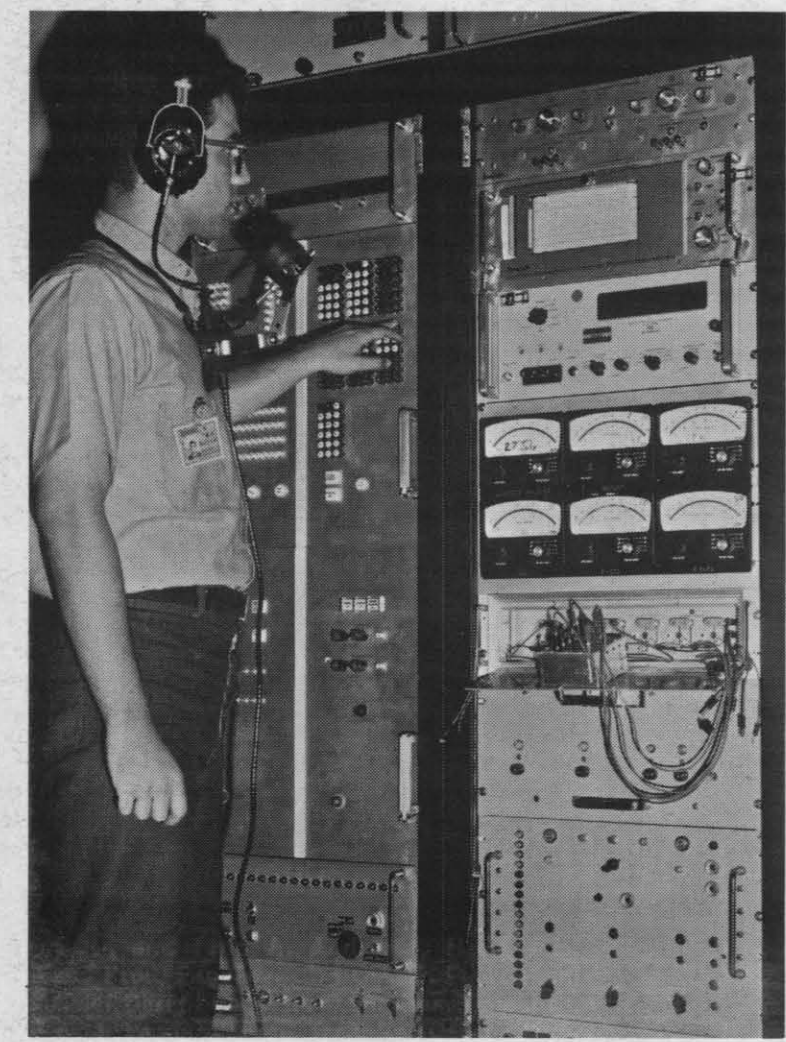
TESTING THE FUNCTIONS of the DASS computer, Data Systems Technician Manuel Menendez uses button panel of DASS's simulator component. DASS translates from digital language of 1218 computer to launcher's analogue lingo.
