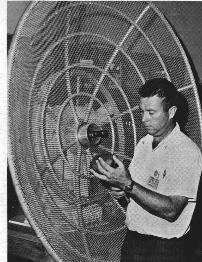
EXAMINING "SPINNER" for installation in former gun antenna is Robert E. Rockwell, Code 30's Instrumentation Lab's Engineering Support Section head. Antenna was for the Army's "sky-sweeper" anti-aircraft gun. It will be converted to a self-controlled receiver for UHF telemetry tests.
