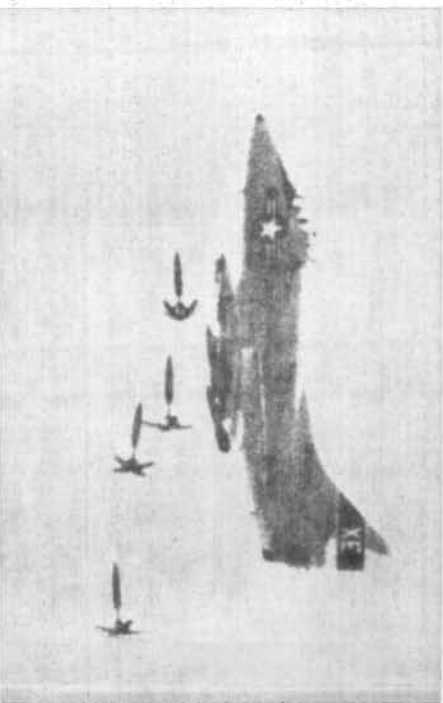
SNAKEY, which employs fins that "blissom out" to retard its trajectory speed, is another NOTS-conceived, designed, developed and tested weapon. Fin device fits either 250 or 500 - pound bombs which can be dropped singly or in multiples.
