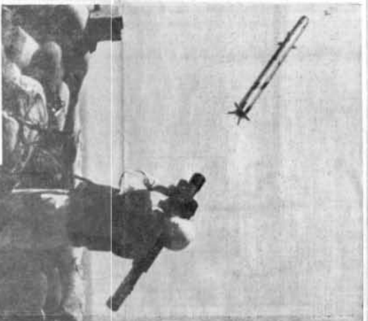
SNAKEY, which employs fins that "blissom out" to retard its trajectory speed, is another NOTS-conceived, designed, developed and tested weapon. Fin device fits either 250 or 500 - pound bombs which can be dropped singly or in multiples.
