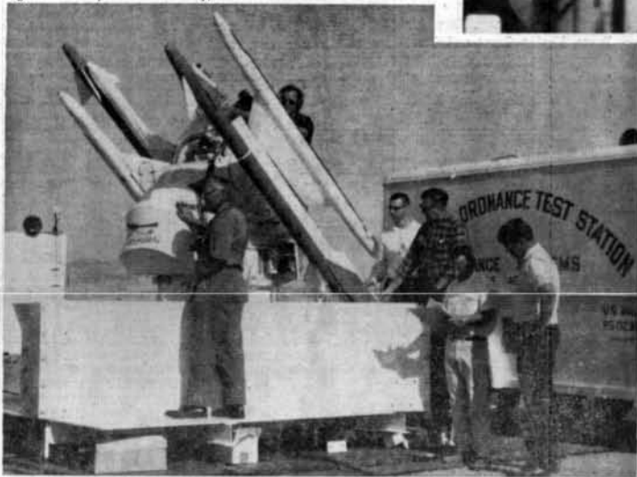
CHAPARAL, an air defense system employing four Sidewinder IC missiles developed here, is undergoing engineering design and evaluation test work under Army sponsor-
