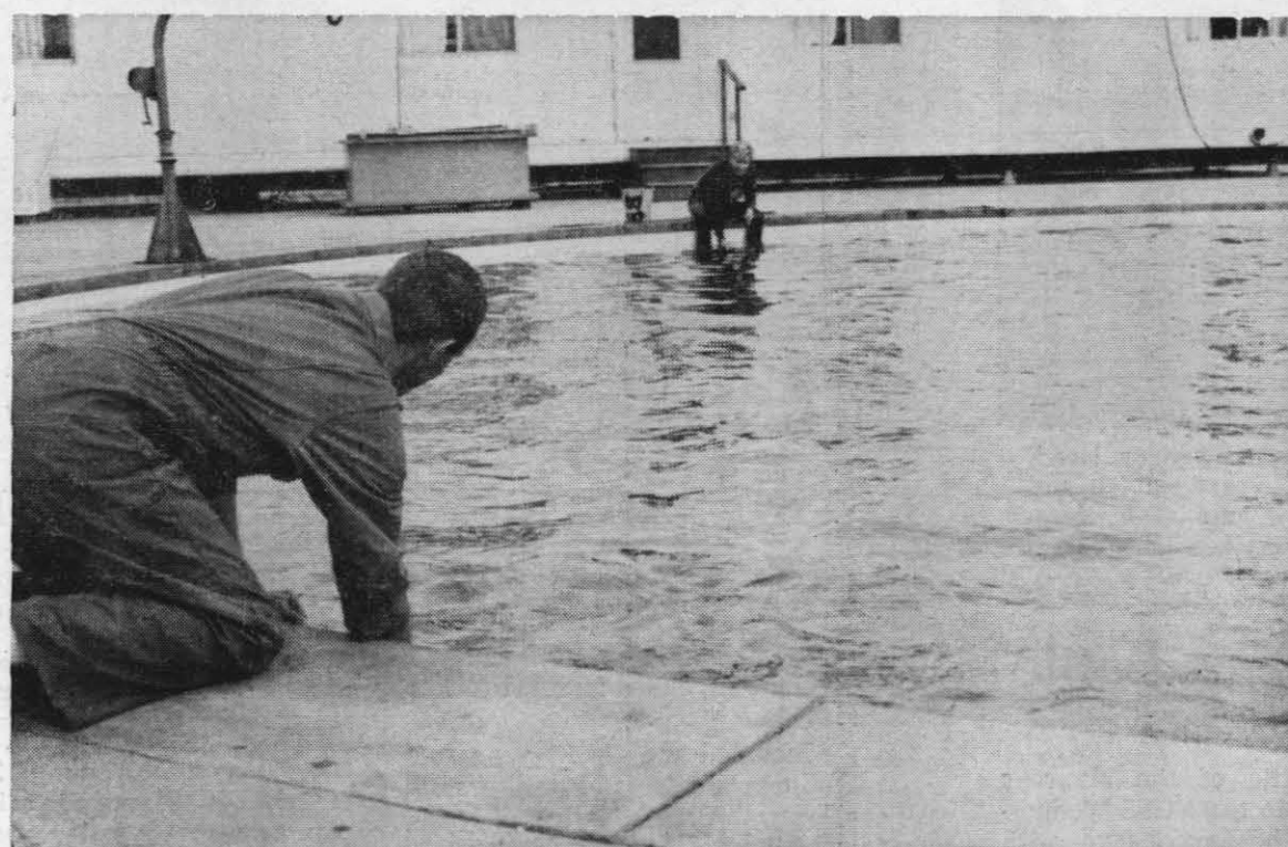
ACOUSTIC "BEACONS," held under water at three stations in pool, command varying actions (above) by "Buzz-Buzz." Bill A. Powell (foreground) and Robert E. Bailey (background) demonstrate application of program.
