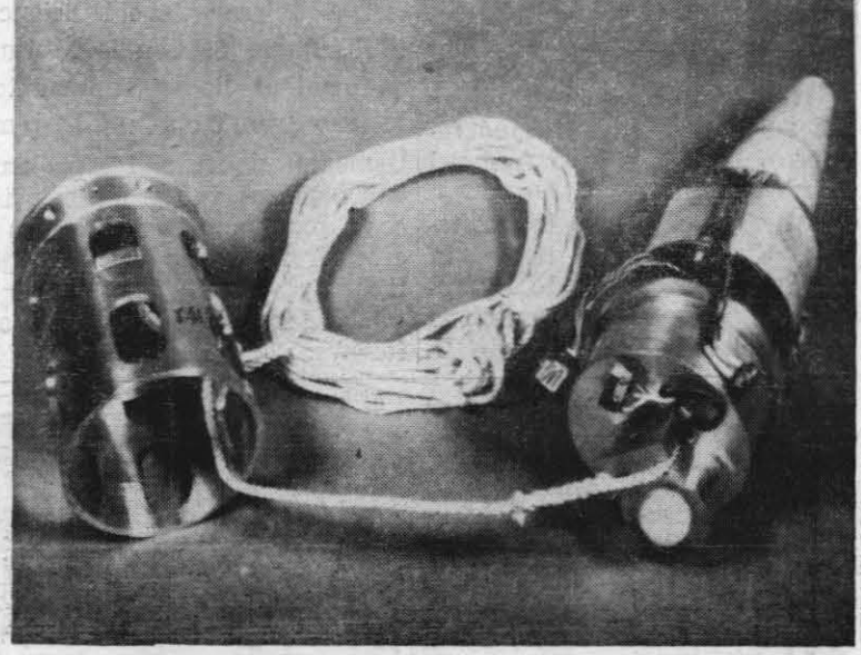
PAYLOAD — High altitude probes will carry this NOTS-developed instrument which will transmit ozone data signals to shipboard receiving equipment as it returns by parachute from a 200,000-ft. altitude.
